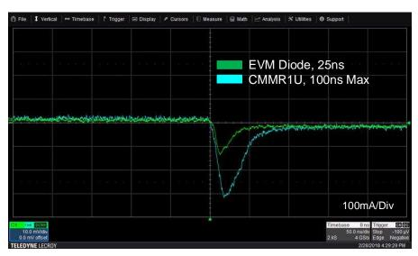
Doubling the recovery time of the EVM diode increased the reverse recovery current three-fold. The CMMR1U diode, rated at 100-ns maximum  $t_{rr}$ , takes only 50 ns to recover, as it is being placed under a different environment from initial tests.
