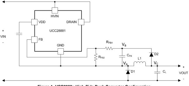
Figure 1. UCC2888x High-Side Buck Converter Configuration
