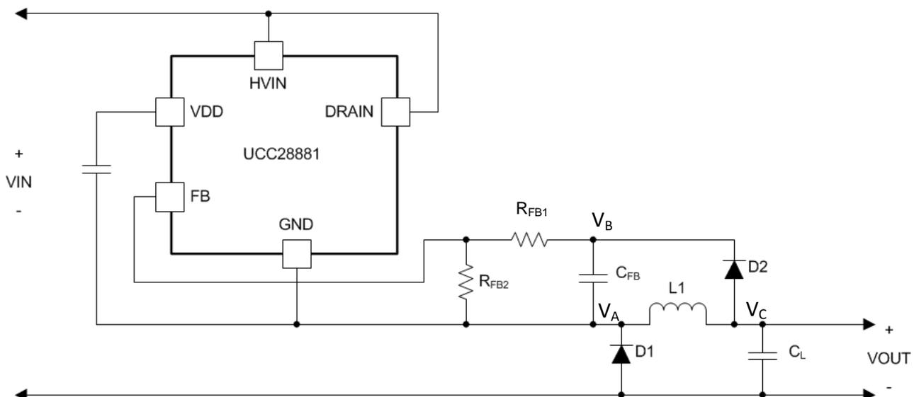
**Figure 1. UCC2888x High-Side Buck Converter Configuration**
