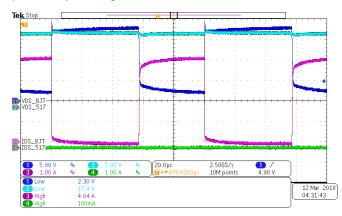
Figure 4. Waveforms of UCC27517 and BJT Totem-Pole Gate Drives at 3.3-V Power Up
