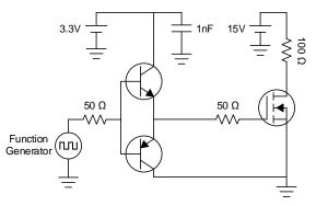
Figure 2. BJT Totem-Pole Schematic
