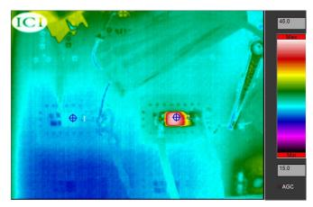
Figure 5. Thermal Image of UCC27517-Driven MOSFET (Left) and BJT-Driven MOSFET (Right) at 3.3-V Power Up
