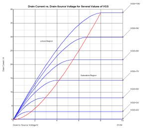
Figure 1. MOSFET IV Characteristics
