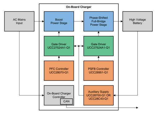
Figure 1. On-Board Charger Block Diagram Example
