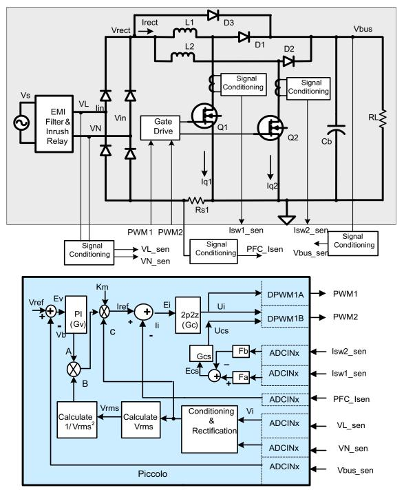
Figure 5. Digital Two-phase Interleaved CCM PFC
