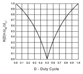
Figure 4. Input Inductor Ripple Current Cancellation
