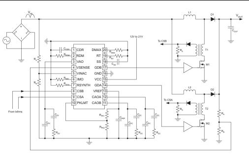
Figure 3. Typical Application Circuit sing the UCC28070-Q1
