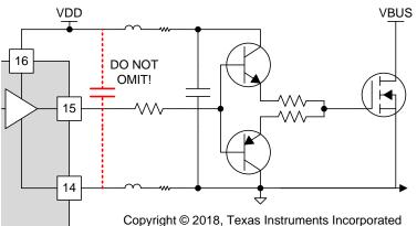
Figure 4. UCC21220 Output Bypassing is Required
