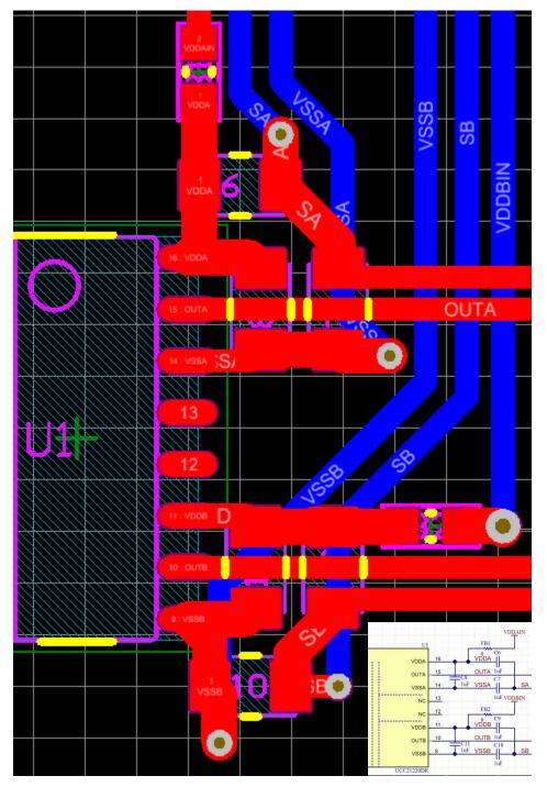
Figure 6. Recommended Placement for Split Capacitor Bypassing with UCC21220
