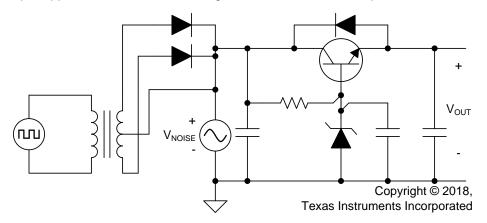
Figure 7. Simple BJT Linear Post-Regulator Circuit
