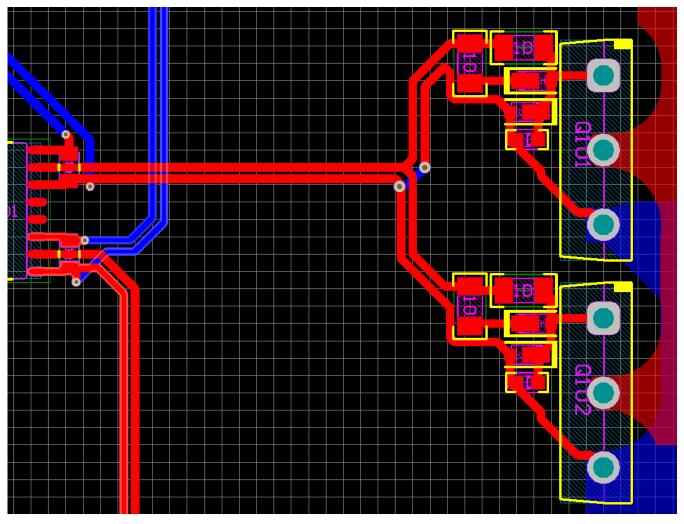
Figure 8. Length Equalization for UCC21220 Driving Two Load Transistors
