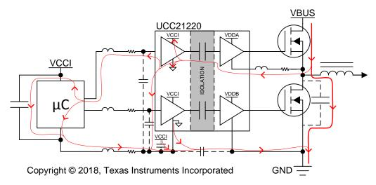
Figure 1. Common-Mode Transient Current Path
