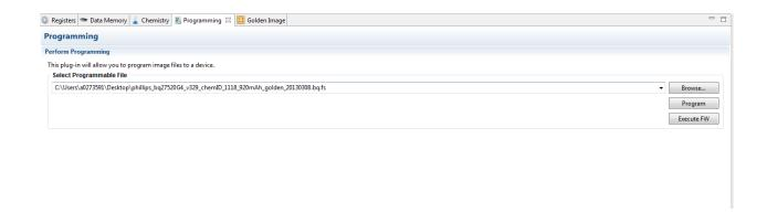
Figure 3. Programming the firmware on the gauge using bqstudio
