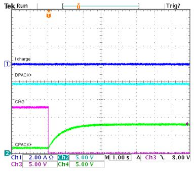
Figure 10. Diode Leakage Example in Hibernate Mode
