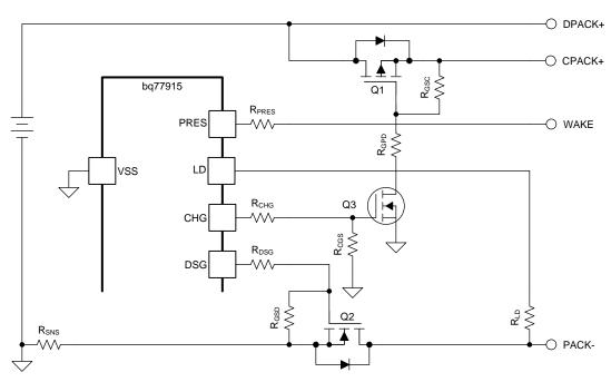
Figure 2. Basic High-side Charge FET
