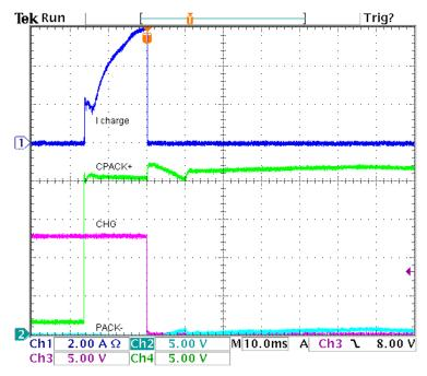
Figure 19. Overcurrent Charge Turn Off
