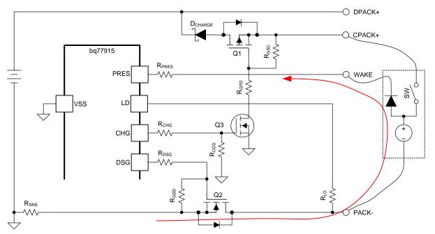
Figure 7. Wakeup From Charger Voltage
