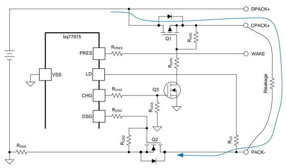
Figure 5. Leakage Into Disabled Charger
