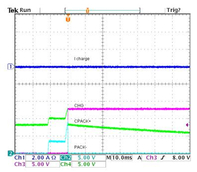
Figure 20. Overcurrent Charge Recovery
