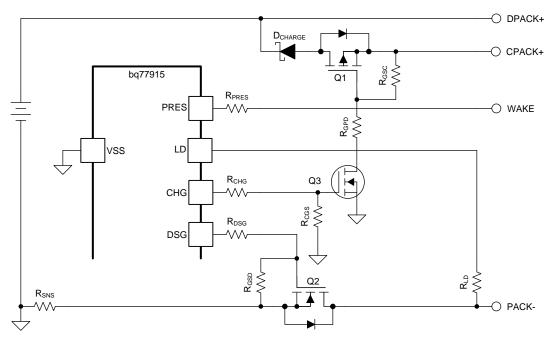
Figure 6. High-side Charge With Diode
