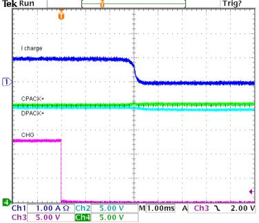
Figure 8. P-channel Resistive Circuit Turn Off
