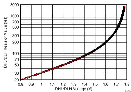
Figure 3. DHL and DLH Pin Voltage Versus Resistor Value
