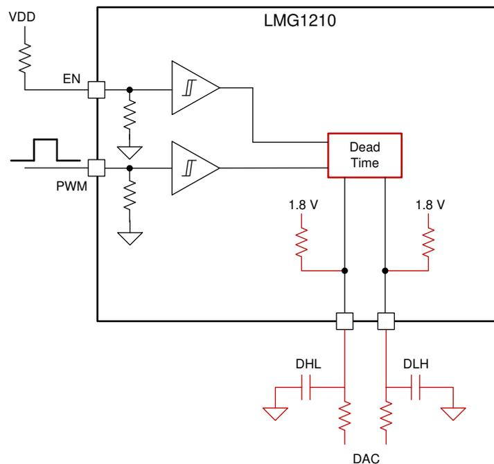
Figure 4. LMG1210 Driving DAC on DHL Pin
