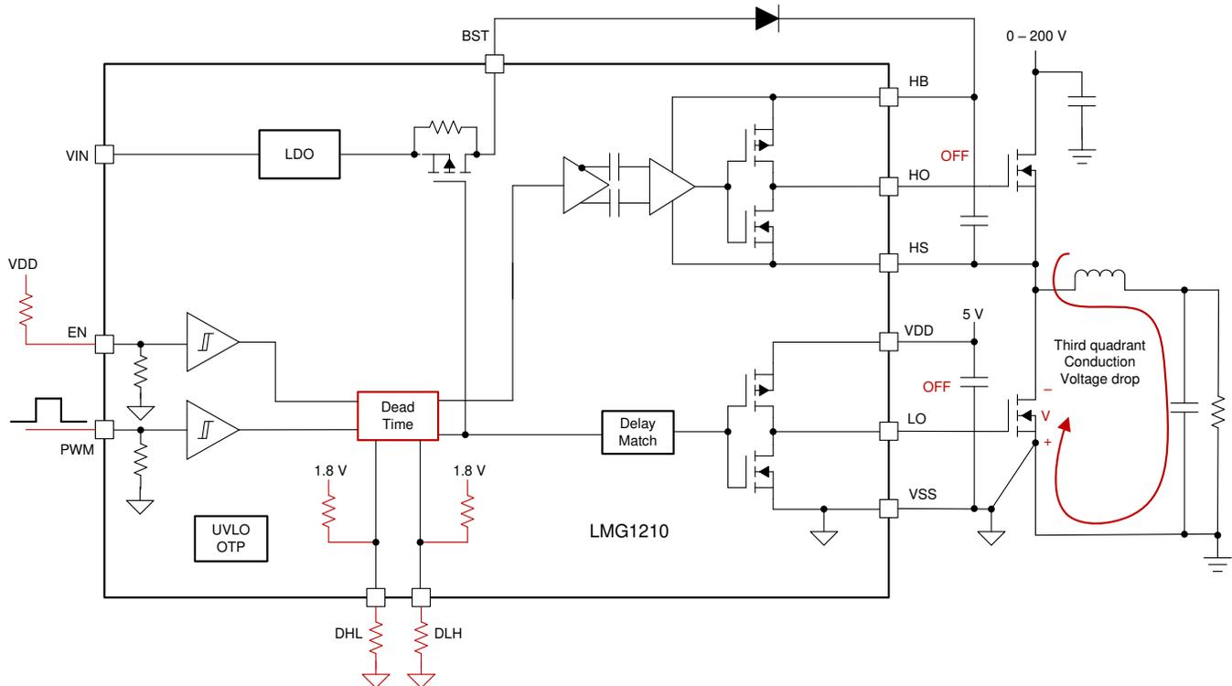
Figure 1. DHL/DLH Pin and Dead-time Conduction Enabled in PWM Mode
