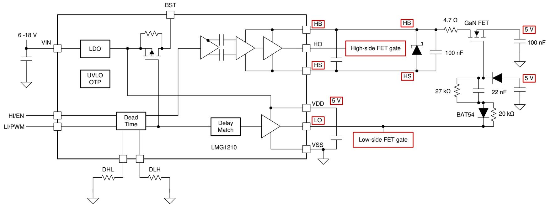
Figure 6. Synchronous Bootstrap Using GaN FET LMG1210 Diagram
