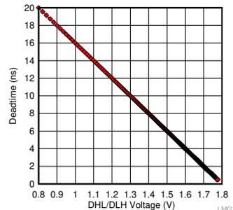
**Figure 5. DHL and DLH Pin Voltage Versus Dead Time**
