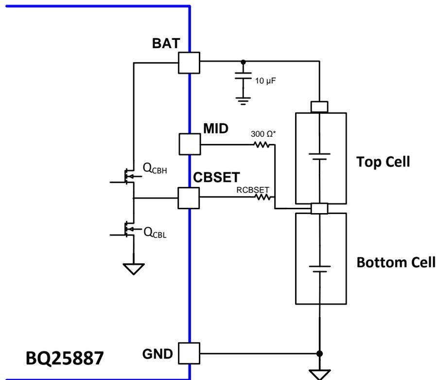
\*Note: The 300-Ω resistor on the MID pin is used to limit the current in cases where the bottom cell is plugged in reversely
