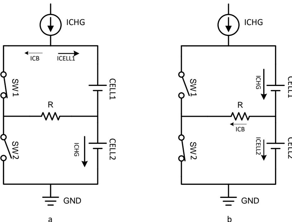
Figure 1. Simplified Cell-Balancing Diagram and Current Illustration Where  $V_{CELL1} > V_{CELL2}$  (a); and  $V_{CELL1} < V_{CELL2}$  (b)
