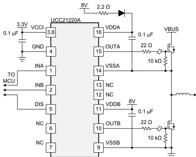
Figure 1. UCC21220A Drives Cascode GaN FETs. Drive Circuit is Similar to Standard MOSFET Circuit.
