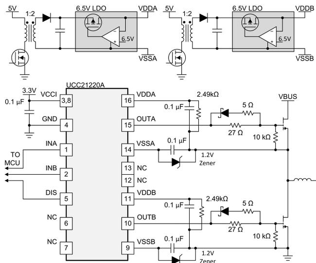
Figure 2. UCC21220A Drives Insulated Gate GaN FETs. Well-regulated Supplies are Required.
