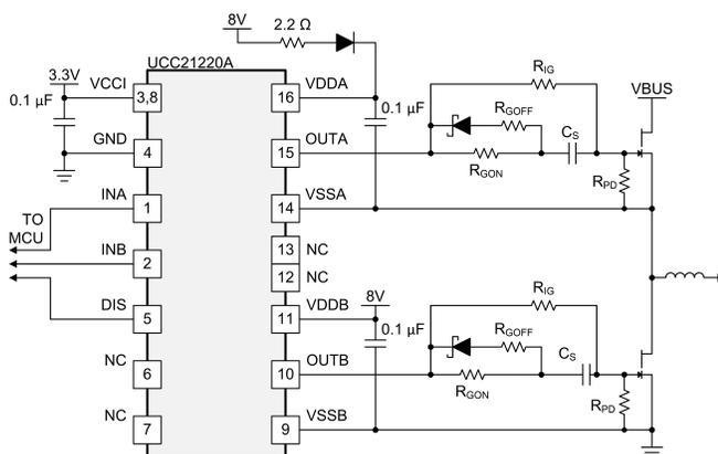
**Figure 3. UCC21220A Drives Non-insulated Gate GaN FETs. Supply Requirements are Relaxed, but the Drive Circuit is Complex.**
