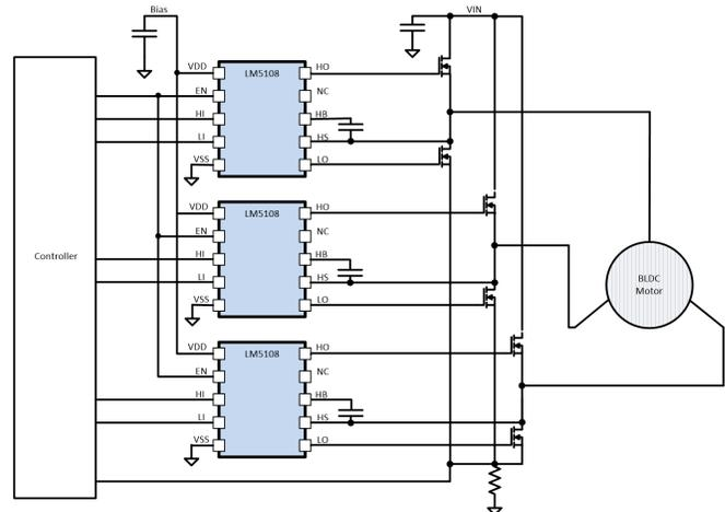
Figure 1. Simplified BLDC Drive with LM5108 Half-Bridge Driver
