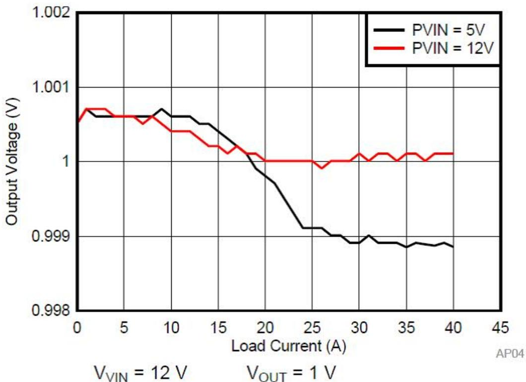
**Figure 1. TPS546D24A Load Regulation**
