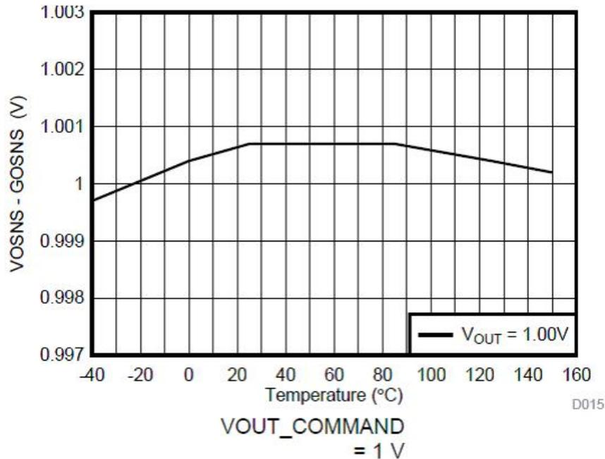
**Figure 2. Output Voltage Versus Junction Temperature**
