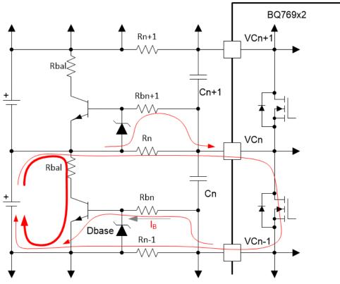
Figure 2-5. Balancing Circuit Using External BJTs
