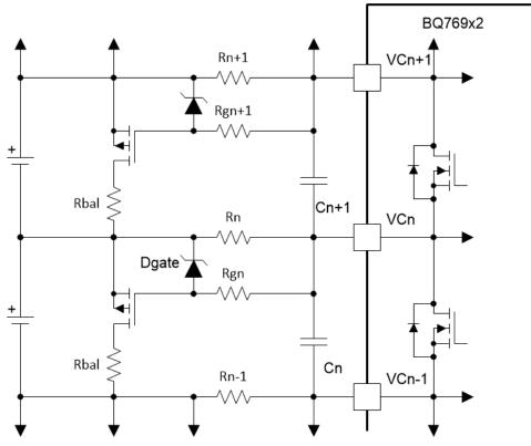
Figure 2-4. Balancing Circuit Using External P-Channel FETs
