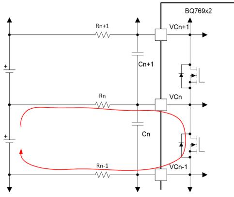
Figure 2-1. Application Circuit for Internal Balancing
