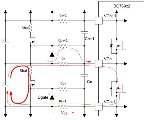
Figure 2-2. Balancing Circuit Using External N-channel FETs
