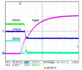
Figure 6-3. Transistor FET Drive, One Discharge FET, On
