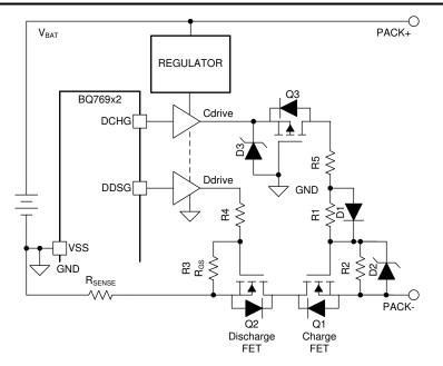
Figure 2-2. Driver with Limited Turn Off Current
