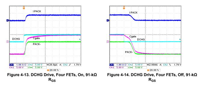
When considering a logic level FET solution a designer should perform a tolerance analysis. With the tolerance on REG1 and the Schottky diode at D3, a sufficiently low  $R_{GSON}$  FET should be used.
