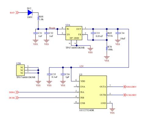
Figure 5-1. IC FET Driver with Regulator Schematic
