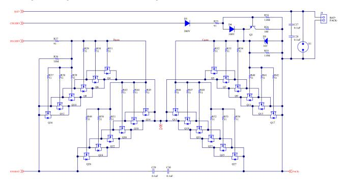
Figure 6-7. Twelve Discharge and Charge FETs Used with Transistor Driver Schematic
