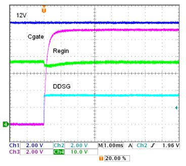
Figure 5-14. 12-V Power When 24 FETs Switch On
