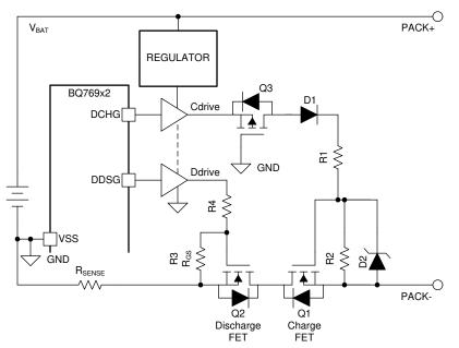
Figure 2-1. Simple Driver Circuit, Resistive Charge Turn Off
