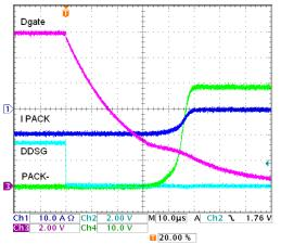
Figure 5-6. IC FET Driver, Four Discharge FETs, Schottky, Off
