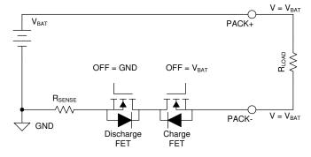
Figure 1-3. Discharge FET Off, Load Attached
