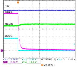
Figure 6-19. 12-V with Push-Pull Driver Turn Off
