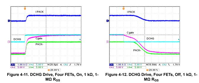
When faster turn off is desired, there is little voltage margin for circuits with the REG1 voltage and logic level FETs. One solution is to use a smaller  $R_{GS}$  resistor R35. Using a 91-k $\Omega$   $R_{GS}$  is shown in Figure 4-13 and Figure 4-14. Turn on is similar to the larger  $R_{GS}$  waveform, while turn off is much faster. With the 5-V supply this solution requires approximately 50  $\mu$ A additional current while the charge FET is on.
