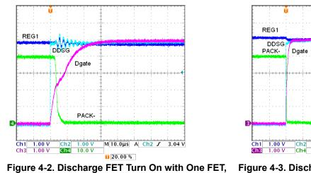
Figure 4-2. Discharge FET Turn On with One FET, 1-kΩ Gate Resistance
