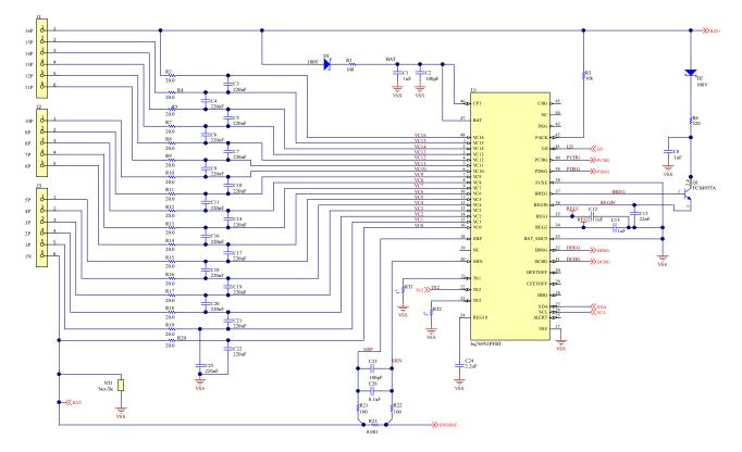
Figure 3-1. BQ76952 Monitor Schematic for Low-Side Switching
