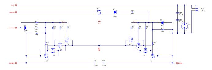
Figure 5-2. Four Discharge and Charge FETs For Driver Schematic
