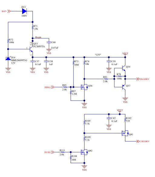
Figure 6-1. Transistor Driver Example Schematic
