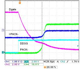
Figure 6-9. Transistor FET Drive, 12 Discharge FETs, Off
