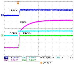
Figure 5-7. IC FET Driver, Four Charge FETs, On
