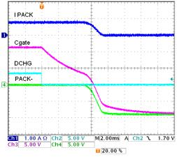
Figure 5-8. IC FET Driver, Four Charge FETs, Off, 91 k $\Omega$
