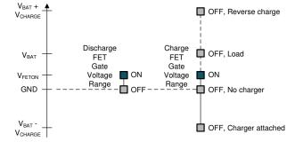
Figure 1-8. Voltage Range for Low Side FET Gates
