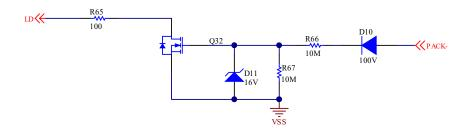
Figure 7-1. LD Circuit for Load Sensing Schematic
