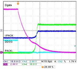
Figure 5-11. IC FET Driver, 12 Discharge FETs, Off
