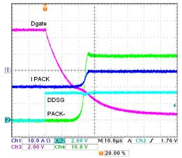
Figure 6-4. Transistor FET Drive, One Discharge FET, Off
