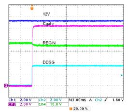
Figure 6-18. 12-V with Push-Pull Driver Turn On
