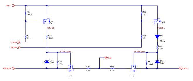
Figure 8-1. Precharge and Predischarge Test Circuit Schematic
