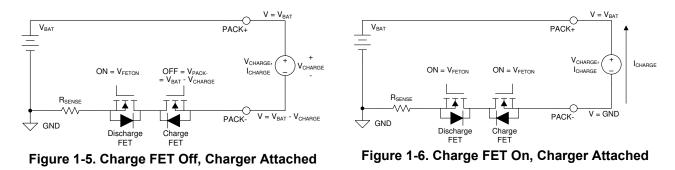
If a reversed charger can be connected to the battery both the battery and charger want to push current in the same direction. Once the fault is detected and the FETs open, the reversed charger pushes the PACK-voltage above the PACK+ voltage. The discharge FET must withstand the high voltage, and the charge FET gate voltage must rise to prevent damage to the FET. This condition is shown in Figure 1-7.
