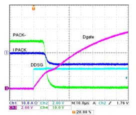
Figure 5-5. IC FET Driver, Four Discharge FETs, Schottky, On
