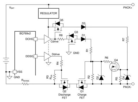
Figure 2-3. Driver with Charge FET Driven Clamp
