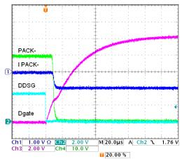
Figure 6-8. Transistor FET Drive, 12 Discharge FETs, On
