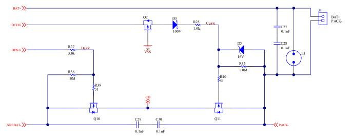
Figure 4-1. DDSG and DCHG as Drivers with Logic Level FETs Schematic
