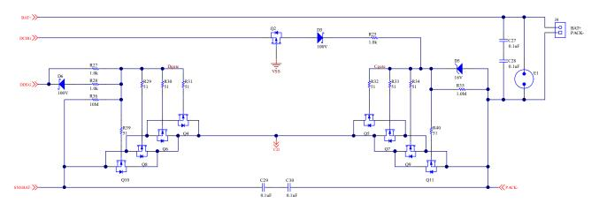
Figure 4-8. DDSG and DCHG as Drivers with Four Logic Level FETs Schematic
