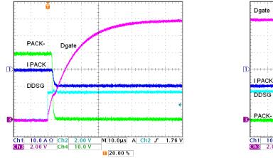
Figure 5-10. IC FET Driver, 12 Discharge FETs, On
