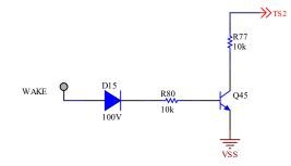
Figure 7-6. Wake Circuit Example Schematic
