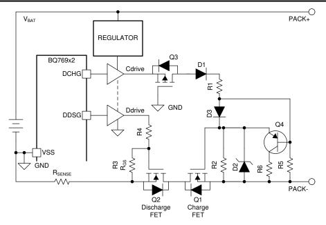
Figure 2-4. Charge FET Driver with PNP Turn Off
