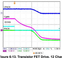
Figure 6-12. Transistor FET Drive, 12 Charge FETs, Figure 6-13. Transistor FET Drive, 12 Charge FETs, Off, PNP, 91 kΩ
