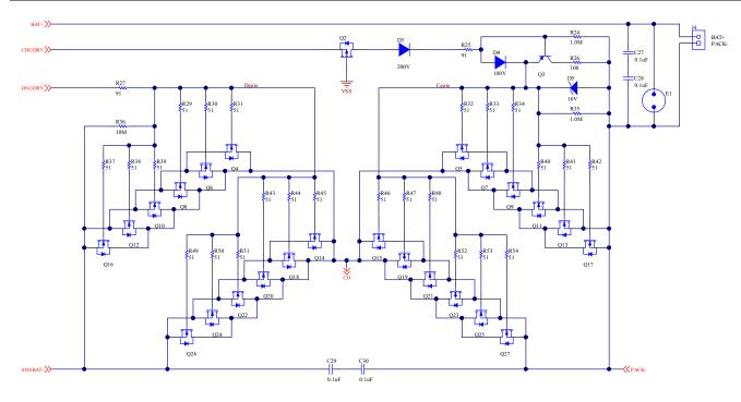
Figure 5-9. 12 Discharge and Charge FETs For IC FET Driver Schematic
