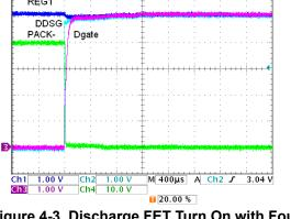
Figure 4-3. Discharge FET Turn On with Four FETs, 1 k $\Omega$ , REG1 Droop
