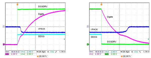
Figure 5-3. IC FET Driver, Four Discharge FETs, On Figure 5-4. IC FET Driver, Four Discharge FETs, Off
