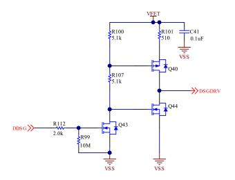
Figure 6-15. Alternate DSG Transistor FET Driver Example Schematic
