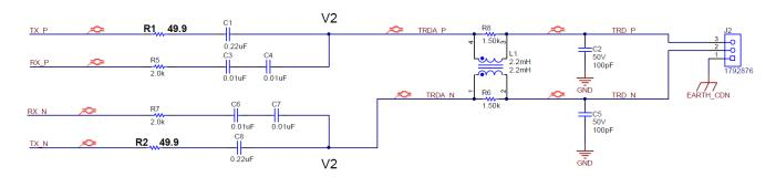
Figure 4-1. 100 ohm Characteristic Impedance Cable Design
