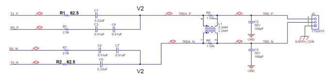
Figure 4-2. 125 ohm Characteristic Impedance Cable Design
