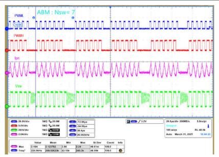
Figure 2-6. ABM Mode PWML Pulse N<sub>SW</sub>=7
