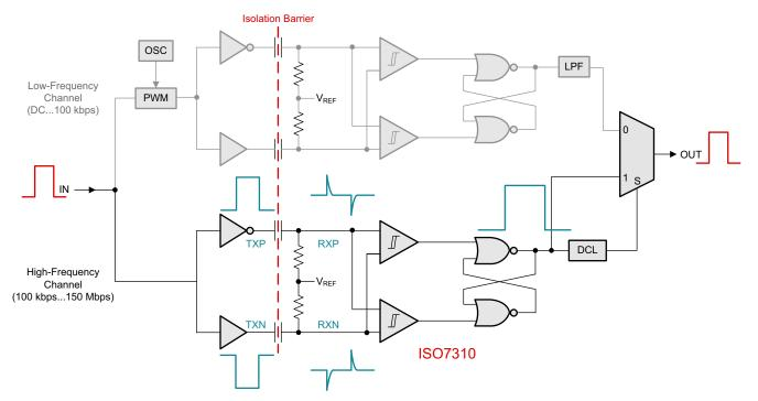
Figure 4-13. Edge Based Isolation Driver Architecture
