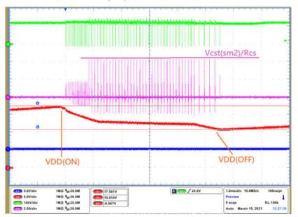
Figure 3-6. SCP Delay to Action
