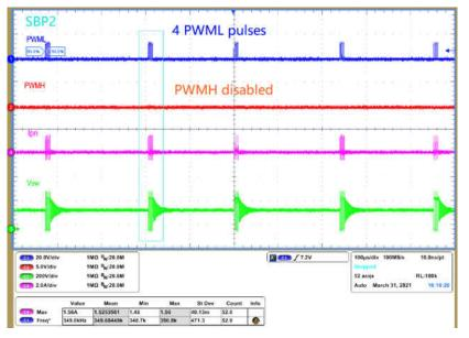
Figure 2-1. SBP2 Mode Operation Waveform
