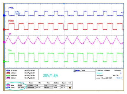
Figure 2-8. AAM Mode Medium Load
