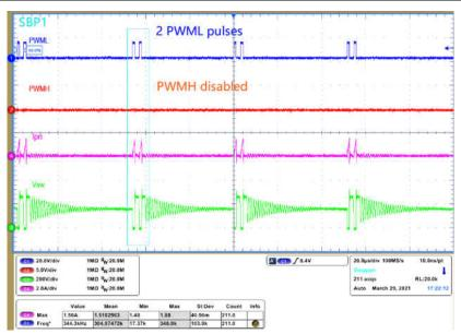
Figure 2-2. SBP1 Mode Operation Waveform
