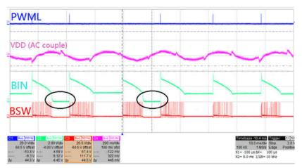
Figure 4-1. Boost Inductor DCR > 1 ohm
