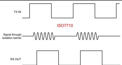
Figure 4-12. Level Based Isolation Driver Architecture
