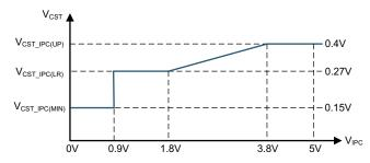
Figure 4-5. IPC Pin Resistor Setting
