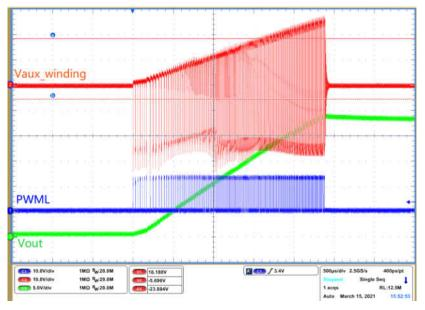
Figure 3-3. OVP Delay to Action
