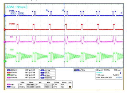
Figure 2-5. ABM Mode PWML Pulse N<sub>SW</sub>=2
