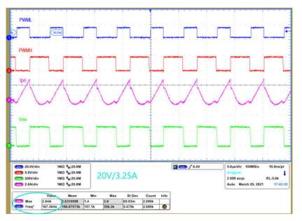
Figure 2-9. AAM Mode Heavy Load
