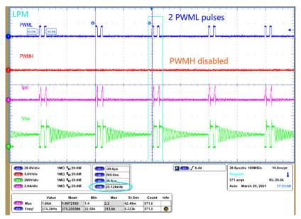
Figure 2-3. LPM Mode Operation Waveform
