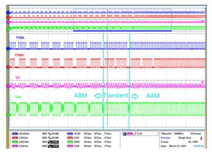
Figure 2-7. ABM to AAM Mode Transition
