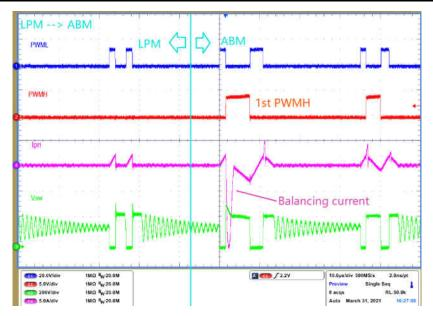
Figure 2-4. LPM to ABM Mode Transition
