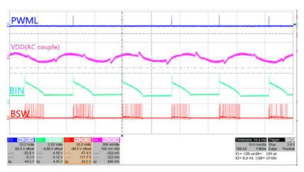
Figure 4-2. Boost Inductor DCR = 0.56 ohm
