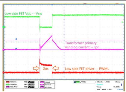
Figure 1-4. CS Pin Fault Detection - Only 1 Pulse With 2us Width
