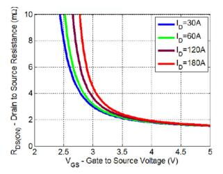
Figure 4. Optimal GaN Drive Voltage
