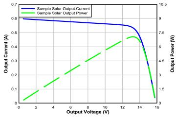
Figure 1-1. Sample I-V and P-V Curve
