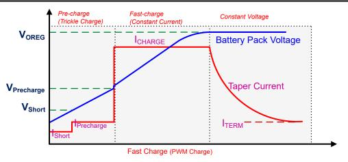
Figure 2-1. Standard CC/CV Charge Profile
