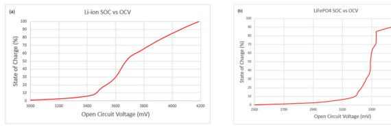
Figure 2-2. Li-ion SOC vs OCV Profiles
