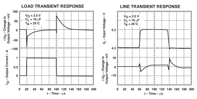
Figure 2. Graphics of Typical Current Transient Response of the 2.5-V Supply Output
