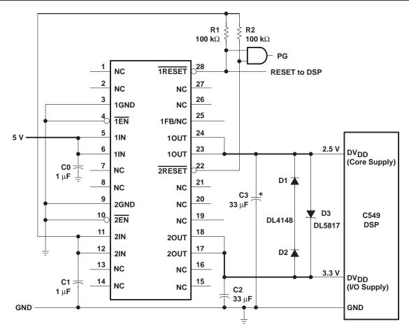
Figure 1. Typical Application Circuit Showing the Suggested Lower Impedance/Wider Copper Supply Lines and Diode Protection
