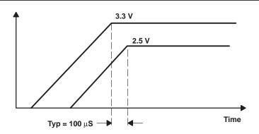
Figure 4. Suggested Power Supply Sequencing of the Core Voltage of 2.5 V and the I/O Voltage of 3.3 V
