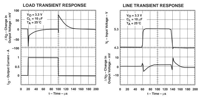
Figure 3. Graphics of Typical Current Transient Response of the 3.3-V Supply Output
