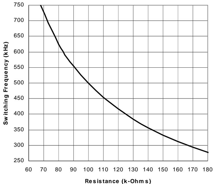
**Figure 2. Switching Frequency Trimming Resistor Selection**
