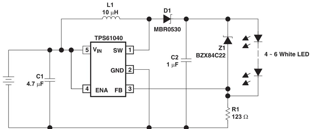
**Figure 1. Constant Current LED Drive Supply**
