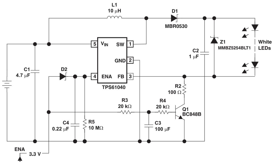
**Figure 2. Additional Components Provide Gradual Turnon and Turnoff of LED Current**
