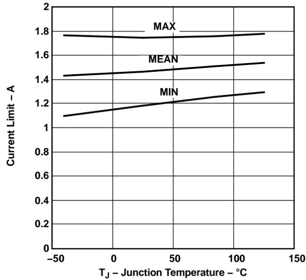
**Figure 5. Statistical Current-Limit Test Results of Power Switch 1**
