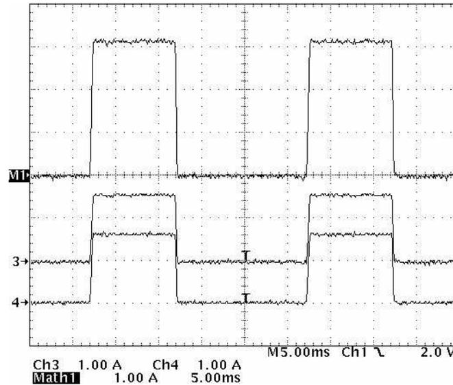
Figure 3. Power Switch in Current Limiting and Thermal Shutdown With  $R_L = 1 \Omega$  (M1:lout; ch3:lout1; ch4:lout2)
