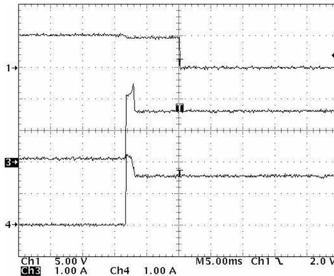
Figure 4. A Overcurrent Load ( $1 \Omega$ ) Connected to Powered Output (ch1: $\overline{OC}$ ; ch3:lout1; ch4:lout2)
