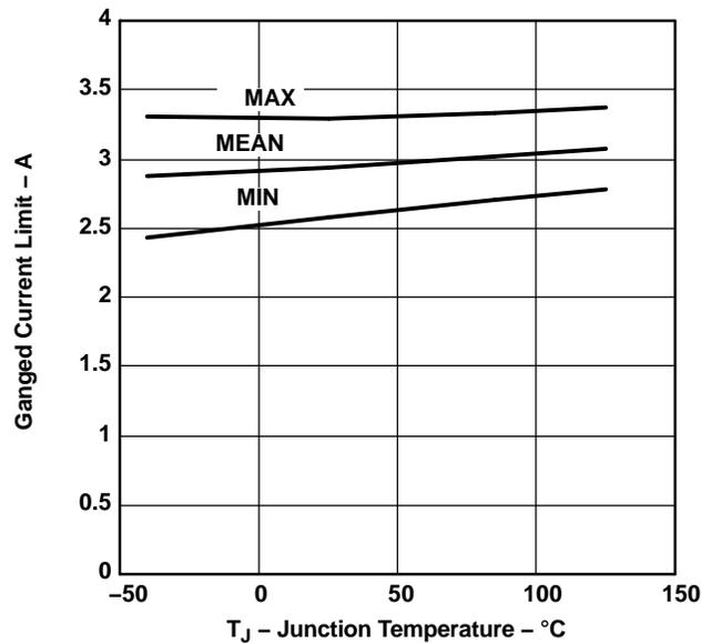
**Figure 7. Statistical Current-Limit Test Results of Ganged TPS2062**
