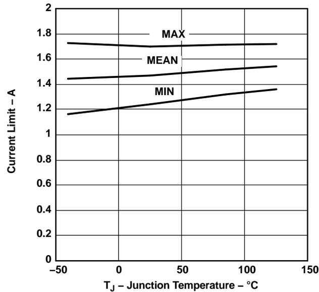
**Figure 6. Statistical Current-Limit Test Results of Power Switch 2**
