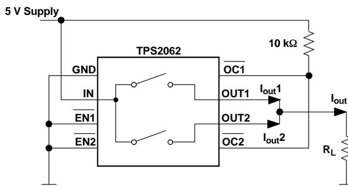
Figure 1. Paralleling Two Power Switches of TPS2062
