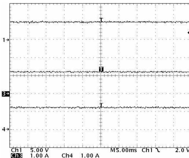
Figure 2. Power Switch Currents With  $R_L = 2 \Omega$  (ch1:OC; ch3:Iout1; ch4:Iout2)
