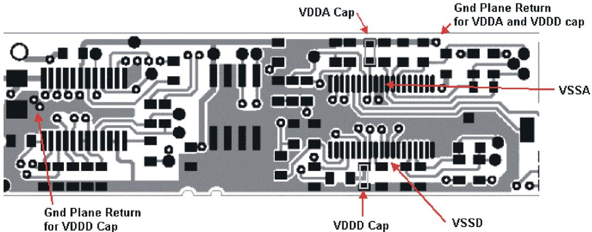
Figure 1. Bad Example of Decoupling Capacitor Placement and Routing
