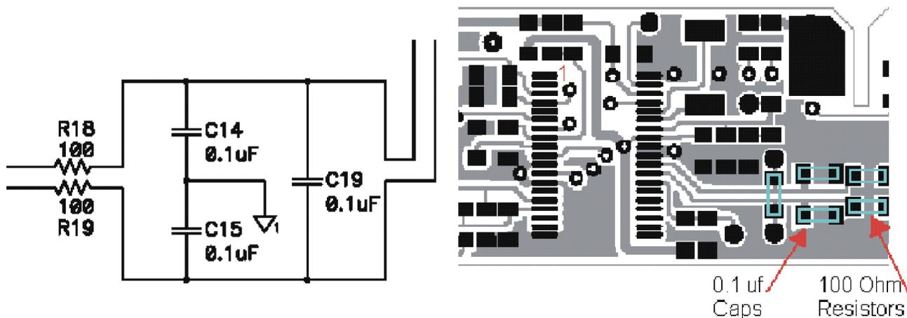
Figure 7. Differential Filter Components With Symmetrical Layout
