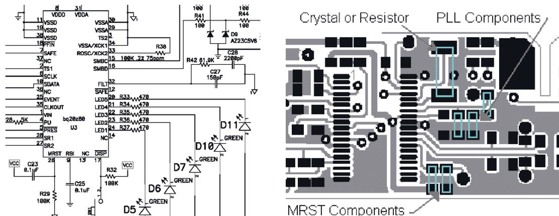
Figure 2. Minimize Length and Loop Area for These Critical Components to Reduce Noise Pickup
