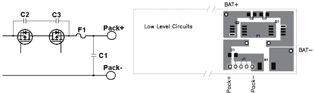
**Figure 3. Use Wide Copper Traces to Lower the Inductance of Bypass Capacitors C1, C2, C3**
