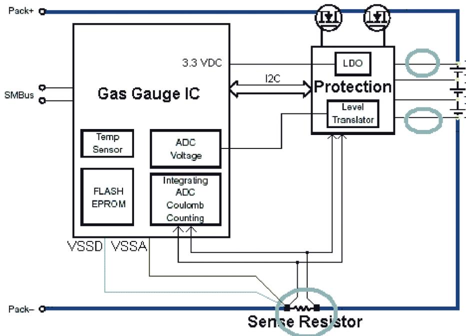
Figure 6. RIGHT! In some cases, top and bottom cell voltage sensing may be extended out to the cells.
