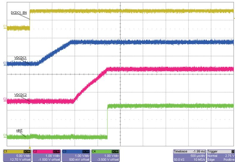
**Figure 6. Scope Trace of  $\overline{\text{INT}}$  Signal for DaVinci™ Reset**
