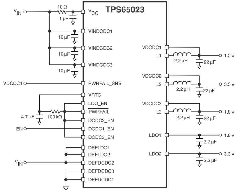
**Figure 3. Sequencing Schematic**
