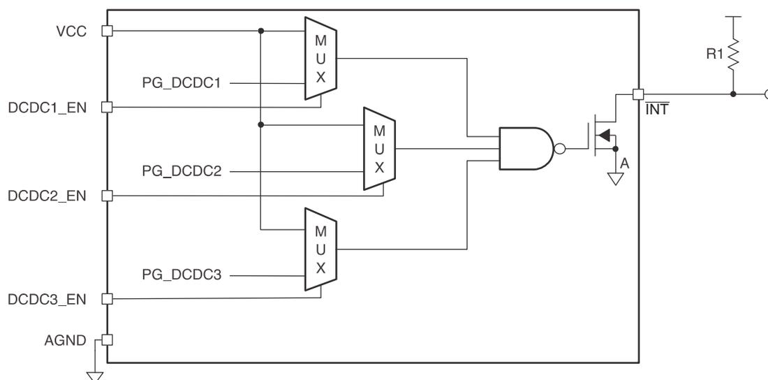
**Figure 2. TPS65023  $\overline{\text{INT}}$  Pin Functional Diagram**
