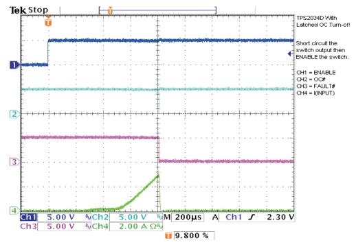
Figure 3. Switch Is Enabled Into Short Circuit
