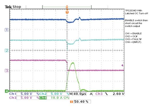
Figure 4. Enabled-Switch Output Is Short Circuited
