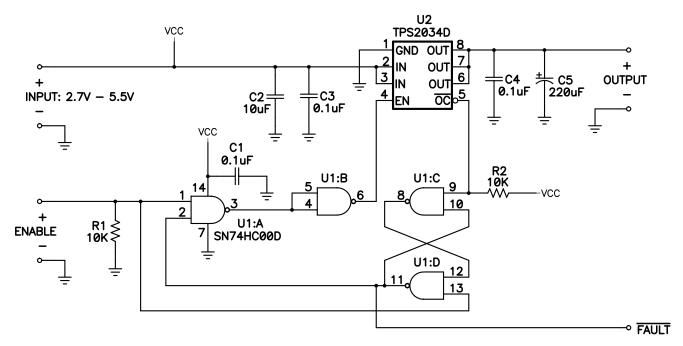
Figure 1. Overcurrent Latch Off Using Quad-NAND Gate
