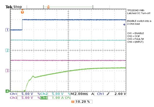
Figure 2. Switch Is Enabled Into 2- $\Omega$  Load
