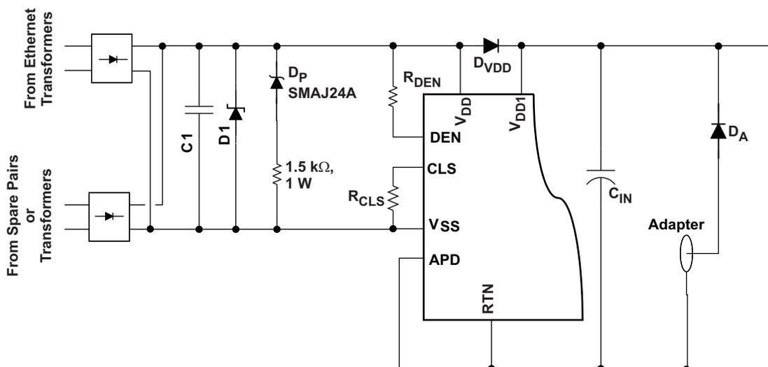
**Figure 11. Keeping the PSE Source On in the Presence of an Adapter Source**
