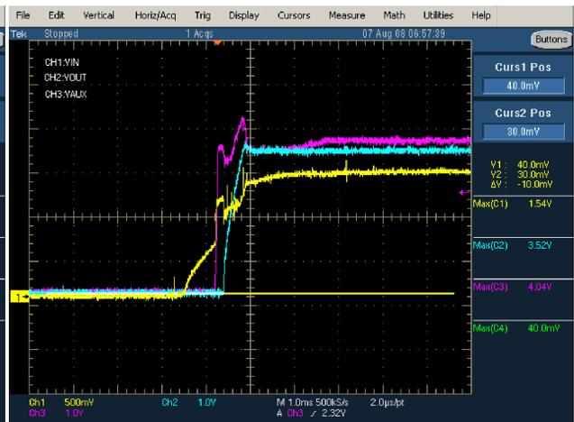
Figure 10. Input and Output Start-Up Voltage Waveform under 1.5-V, 100-mA Conditions
