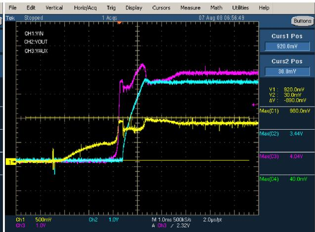
Figure 8. Input and Output Start-Up Voltage Waveform under 0.9-V, 100-mA Conditions
