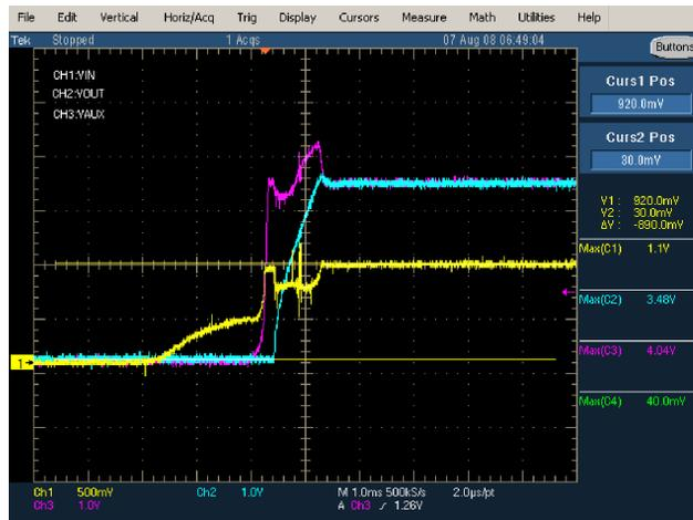
Figure 7. Input and Output Start-Up Voltage Waveform under 0.9-V, 30-mA Conditions
