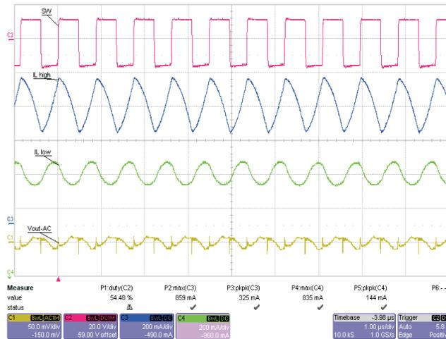
Figure 8. Operation Including  $V_{RIPPLE}$  at  $V_{IN} = 15\text{ V}$  and  $I_{OUT} = 800\text{ mA}$
