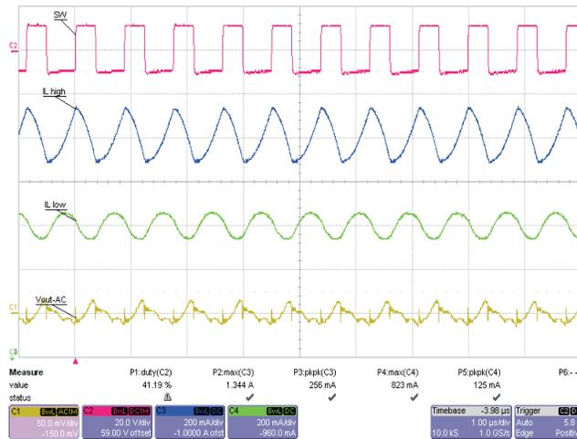
Figure 7. Operation Including  $V_{RIPPLE}$  at  $V_{IN} = 9\text{ V}$  and  $I_{OUT} = 800\text{ mA}$
