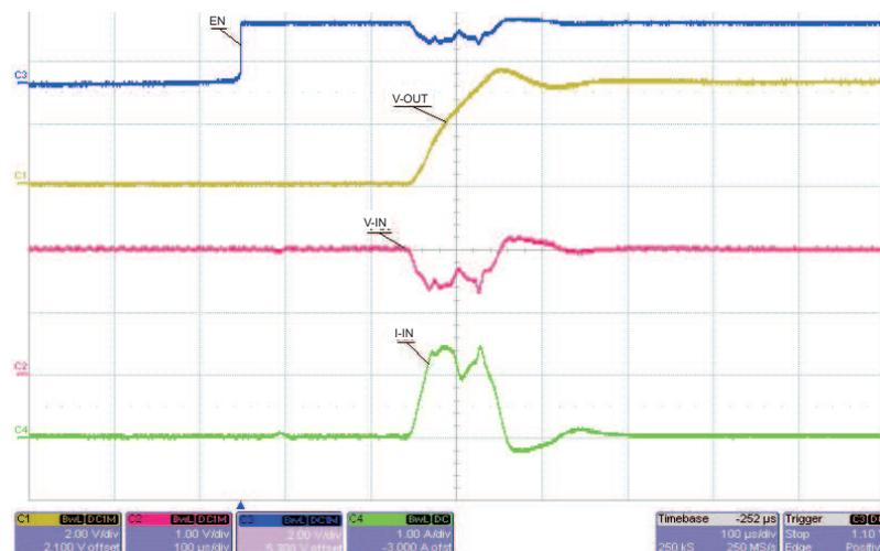
Figure 1. Standard Boost Converter Without Controlled Start-Up
