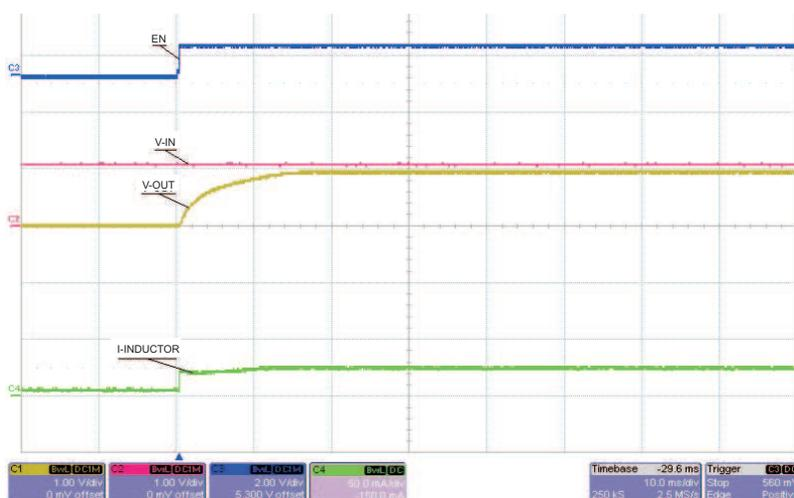
**Figure 8. TPS61020 Start-Up Stuck in Precharge, Load 45  $\Omega$**
