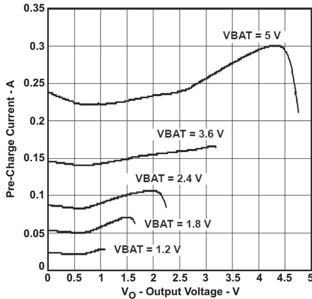
Figure 3. Short-Circuit Precharge Current
