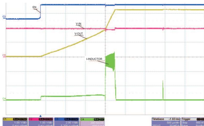
**Figure 5. TPS61020 Start-Up From 2 V**
