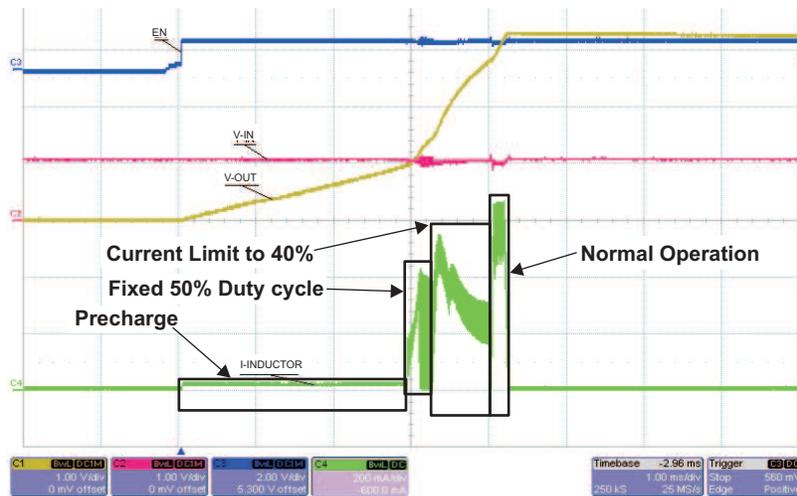
Figure 4. TPS61020 Start-Up From 1 V
