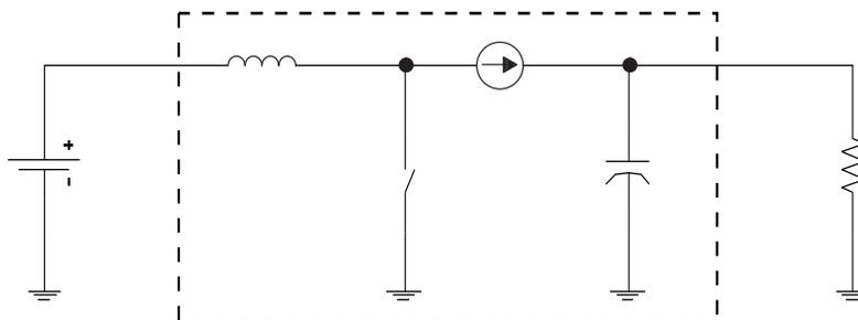
**Figure 7. Configuration for Precharge**
