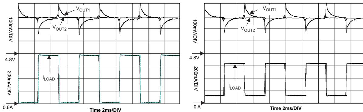
Figure 13. Isolated vs Non-isolated Transient Response
