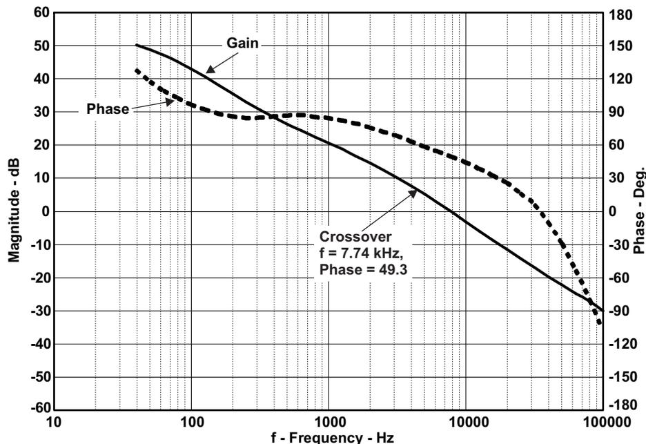
Figure 7. Isolated Circuit Phase/Gain
