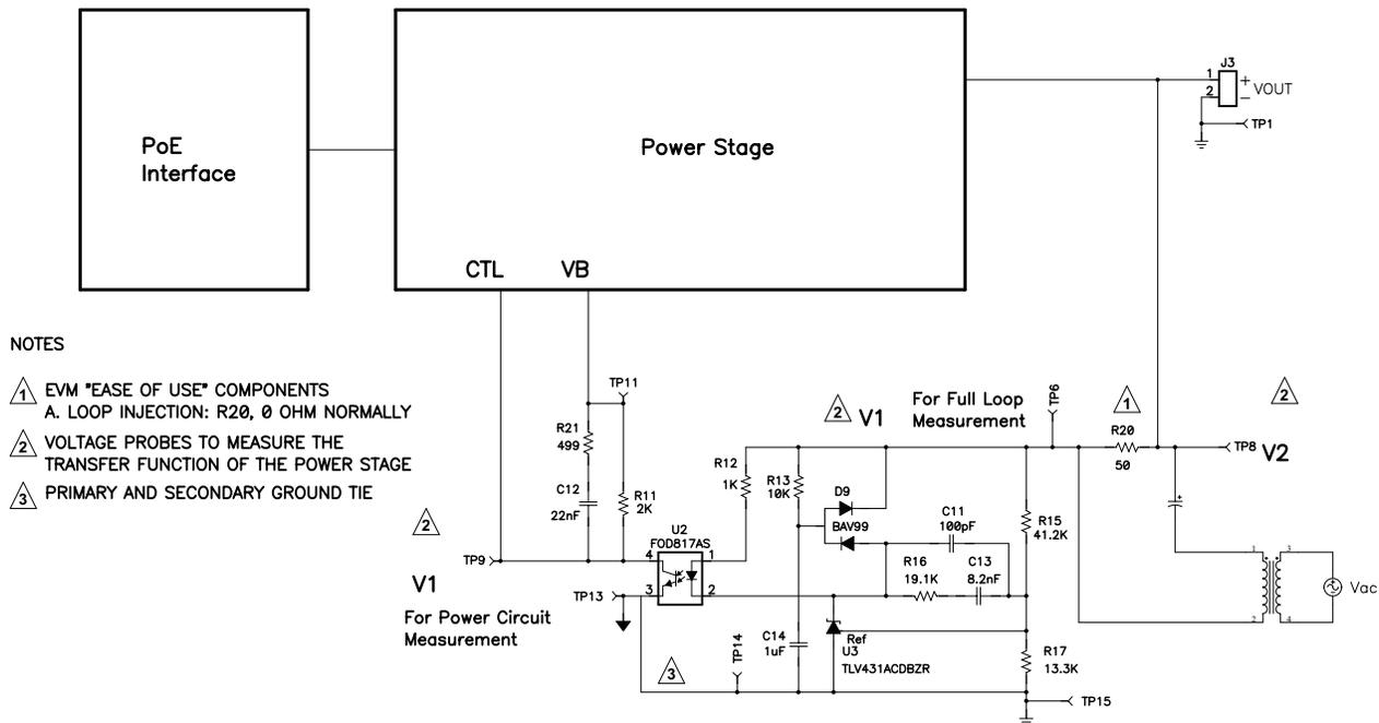
Figure 6. Setup for EVM Phase/Gain Measurement
