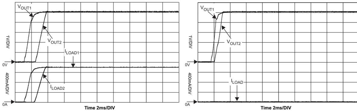
**Figure 14. Isolated vs Non-isolated Circuit Startup**
