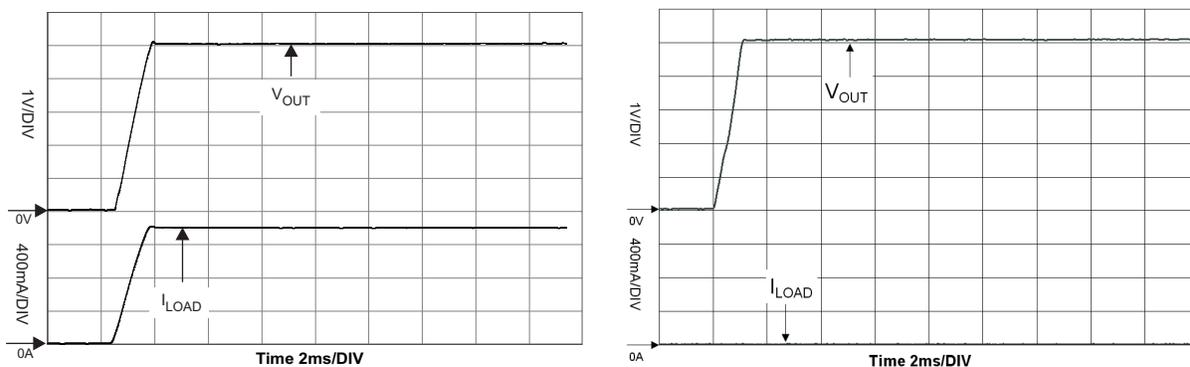
Figure 11. Non-isolated Circuit Startup
