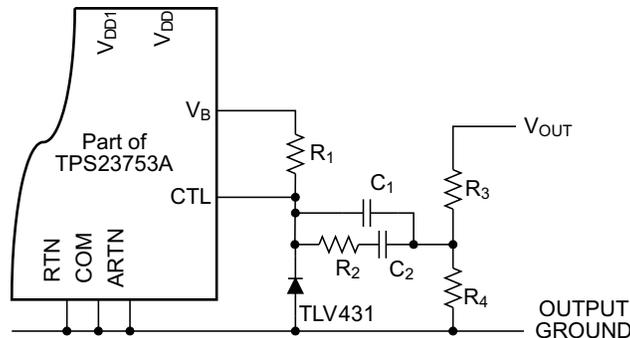
Figure 8. TL431 Error Amplifier Direct Interface
