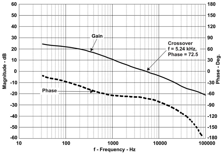
Figure 4. Power Stage Phase/Gain
