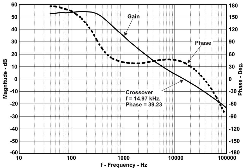
Figure 12. Non-isolated Circuit Phase/Gain
