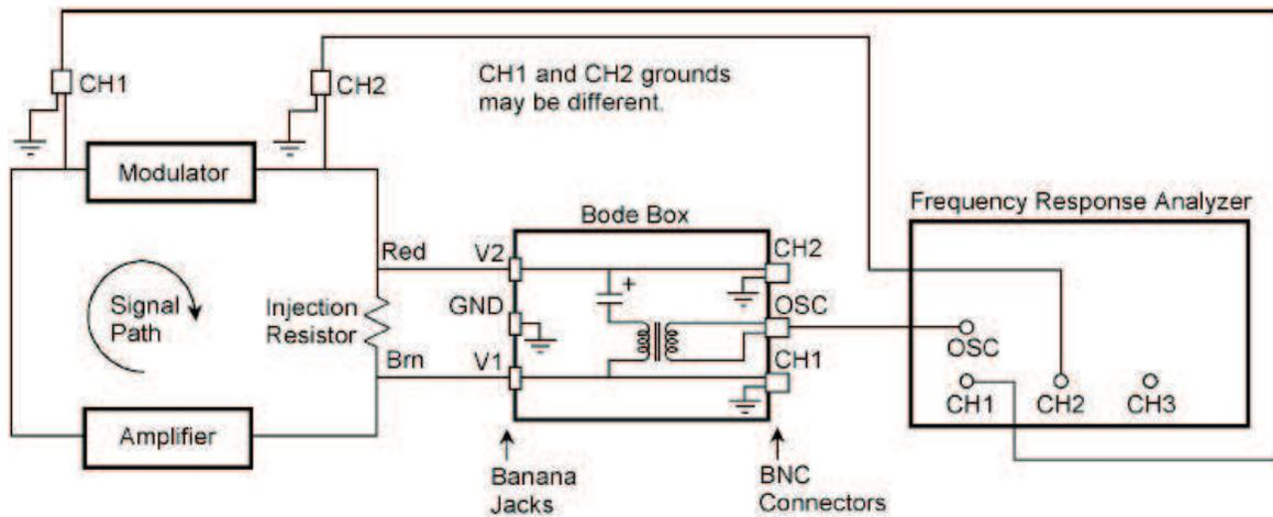
Figure 5. Set up for the Power Stage Phase/Gain Measurement Using the Venable Windows Software 4.0 For MODEL 3120, Venable Instruments®, 2006
