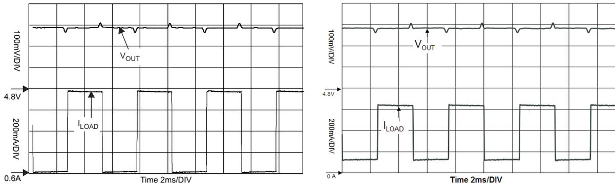
Figure 10. Non-isolated Circuit Transient Response
