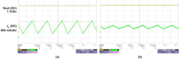
Figure 4. TPS62150 Output Voltage Regulation With (a) 0.47-µH and (b) 2.2-µH Inductor
