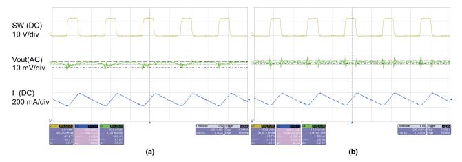
Figure 5. Output Voltage Ripple With 4.7-µH Inductor and (a) 10-µF and (b) 100-µF Capacitors
