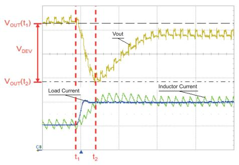
Figure 1. Load Transient Response of the TPS62130
