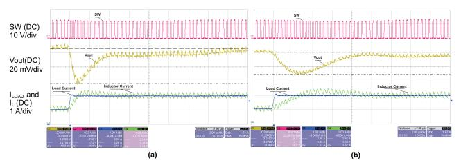
Figure 2. Load Transient With 2.2-µH Inductor and (a) 10-µF and (b) 100-µF Capacitor
