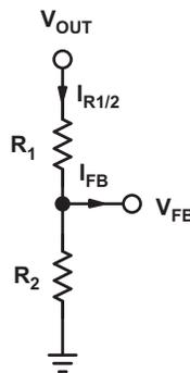
**Figure 2. Resistive Divider for Setting the Output Voltage**
