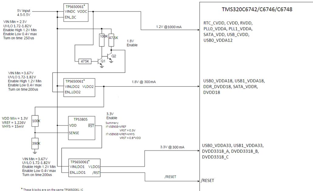
Figure 1. TPS3805, TPS650061, and TMS320C6742/C6746/C6748 Block Diagram
