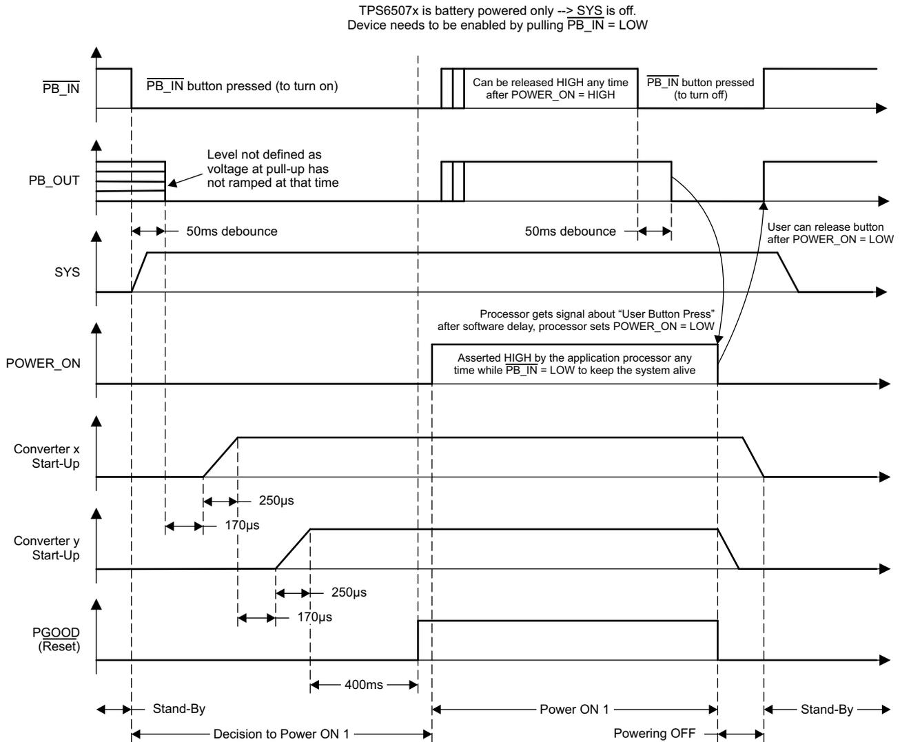
**Figure 3. Case A - Battery Powered (No AC or USB Input Voltage)**
