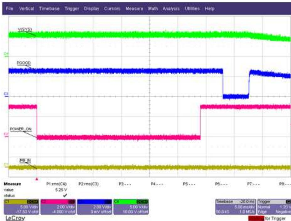
Figure 8. POWER\_ON Triggers “Powering OFF” State, PGOOD and SYS Signals Start to Ramp Down
