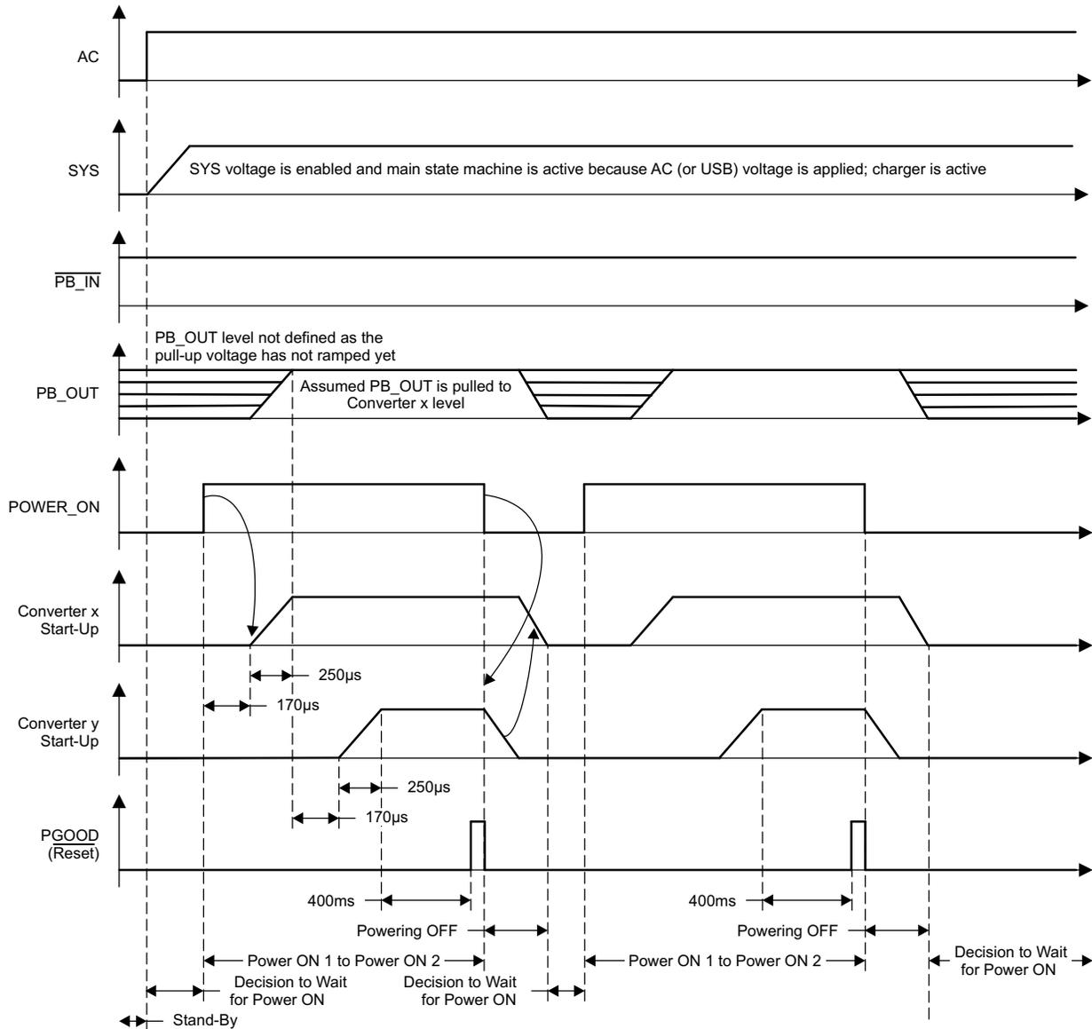
Figure 5. Case C – AC or USB Powered
