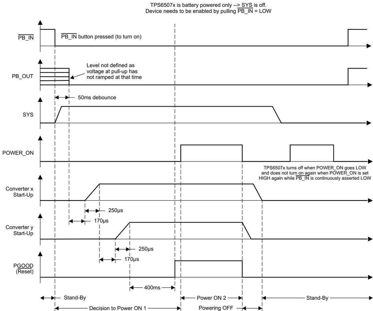
**Figure 4. Case B - Battery Powered (No AC or USB Input Voltage)**
