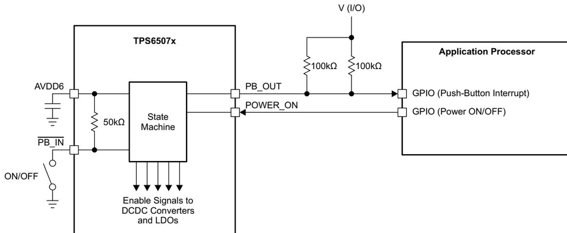
**Figure 1. Block Diagram of TPS6507x and Application Processor System**
