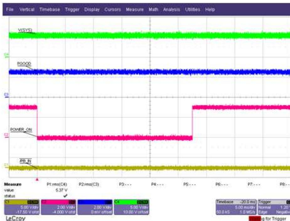
Figure 7. POWER\_ON Fails to Trigger “Powering OFF” State
