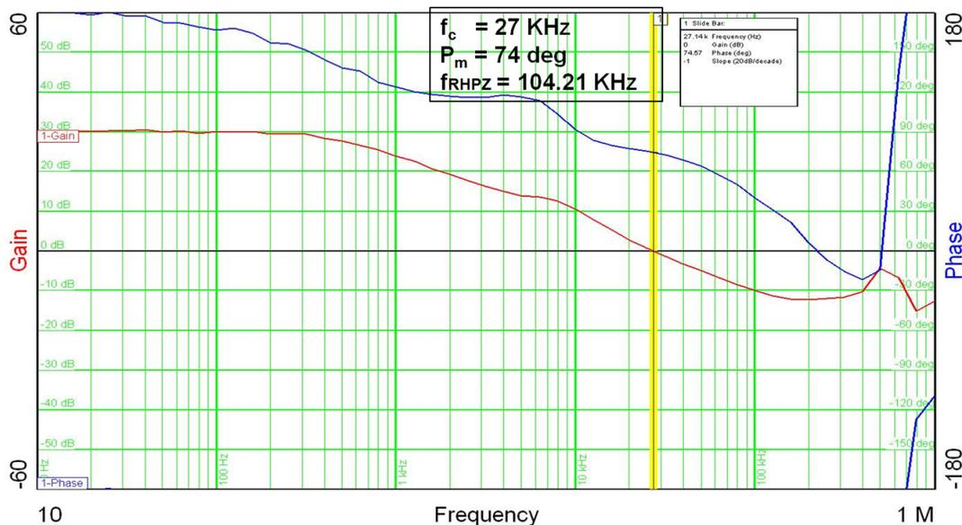
Figure 15. Bode Plot with  $V_{\text{IN}} = 5 \text{ V}$  and 120-mA Load
