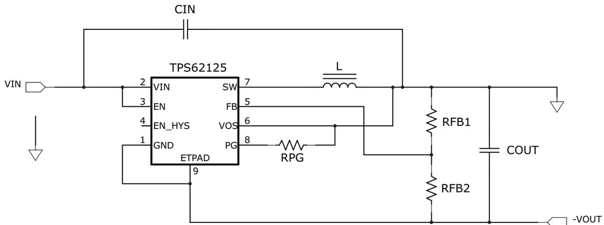
**Figure 2. TPS62125 Inverting Buck-Boost Topology**
