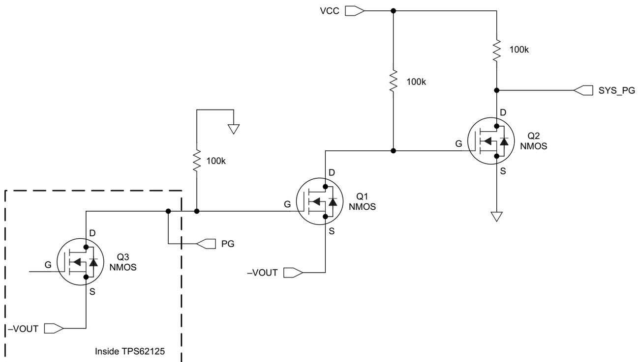
**Figure 8. PG Pin Level Shifter**
