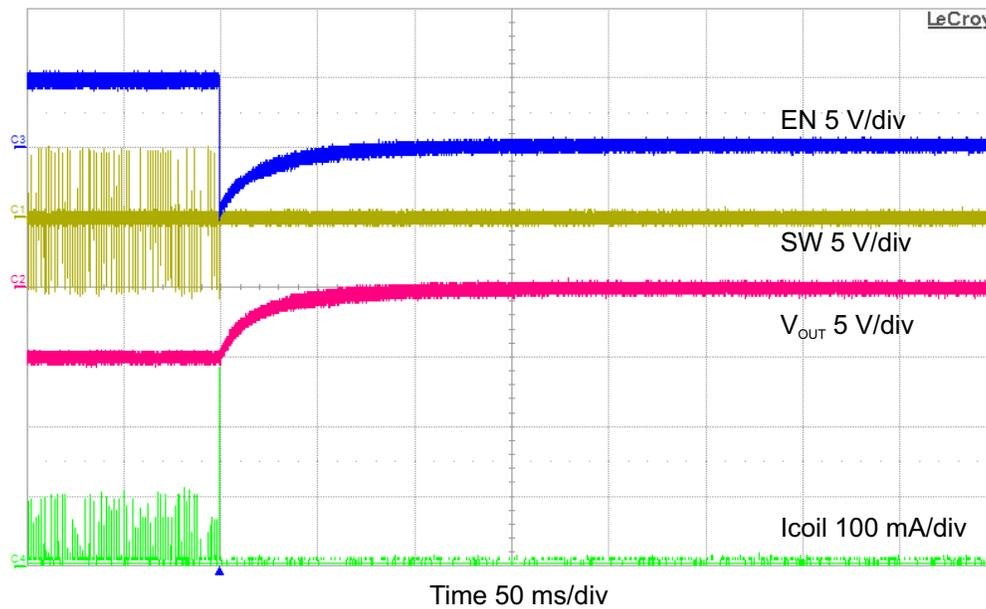
**Figure 12. Shutdown at No Load and PG Pin Discharge of 100 Ohm**
