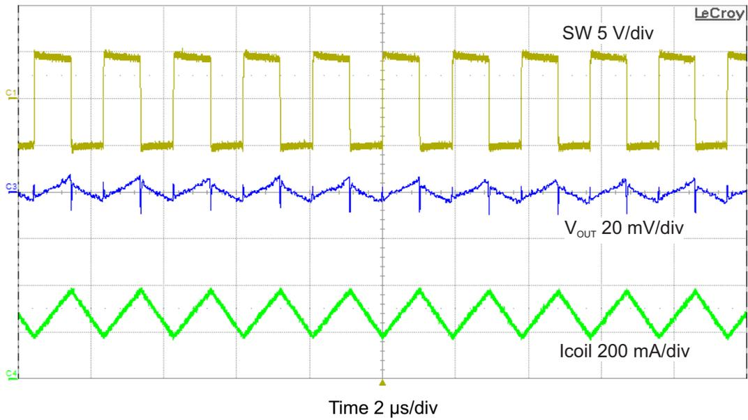
Figure 22. Output Voltage Ripple with  $V_{IN} = 5\text{ V}$  and 120-mA Load
