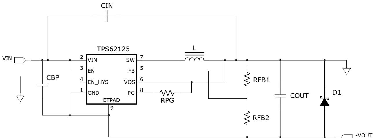
**Figure 14. If Installing CBP, Installing Schottky D1 is Required**
