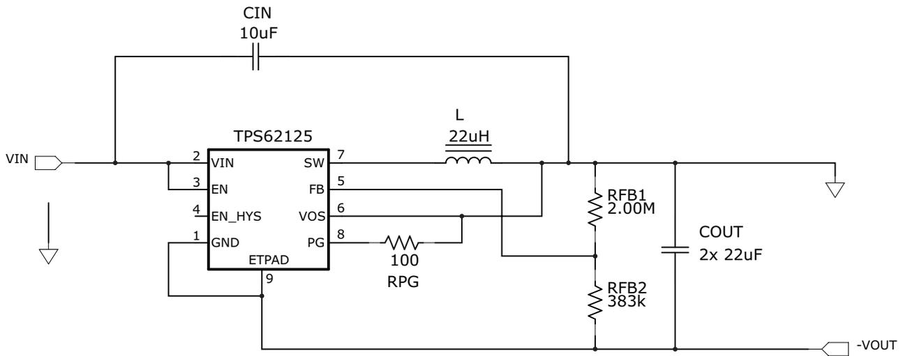
Figure 16. Schematic of the Tested Circuit
