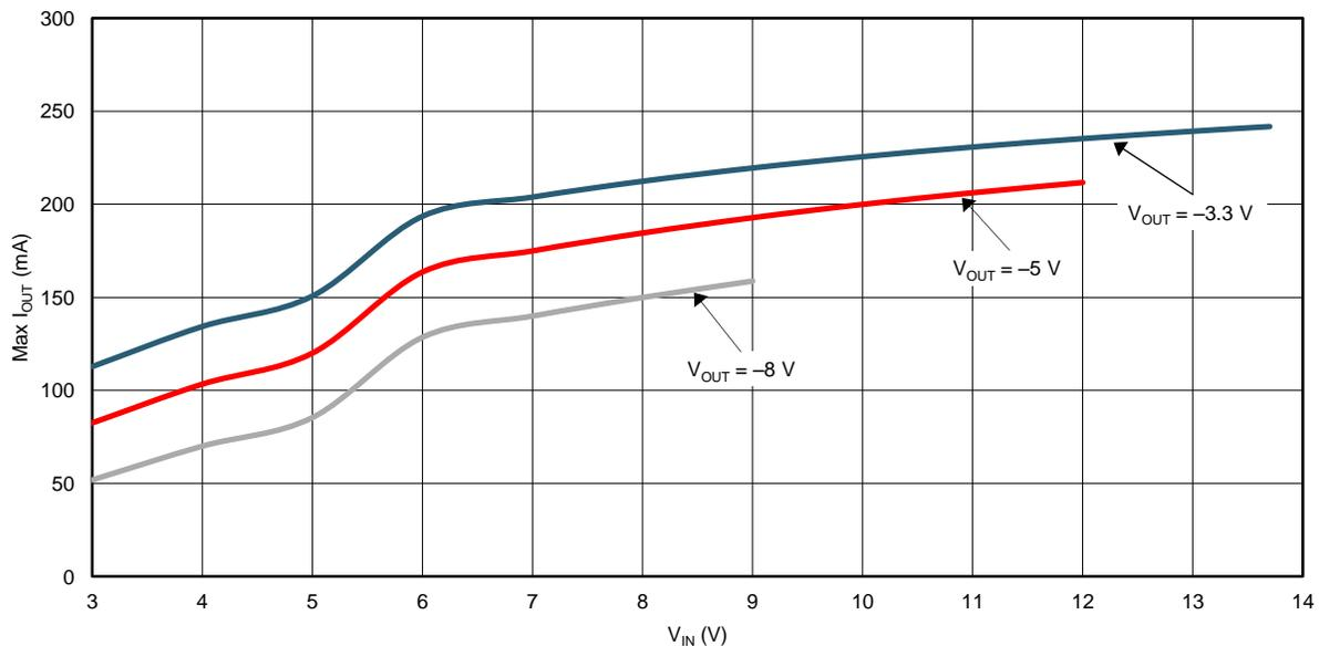
**Figure 4. Maximum Output Current versus Input Voltage**
