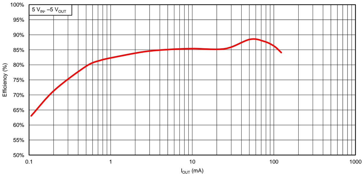
Figure 17. Efficiency versus Load Current with  $V_{OUT} = -5$  V
