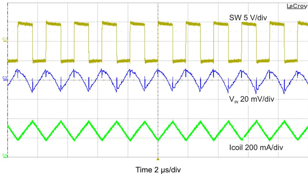
Figure 21. Input Voltage Ripple with  $V_{IN} = 5\text{ V}$  and 120-mA Load
