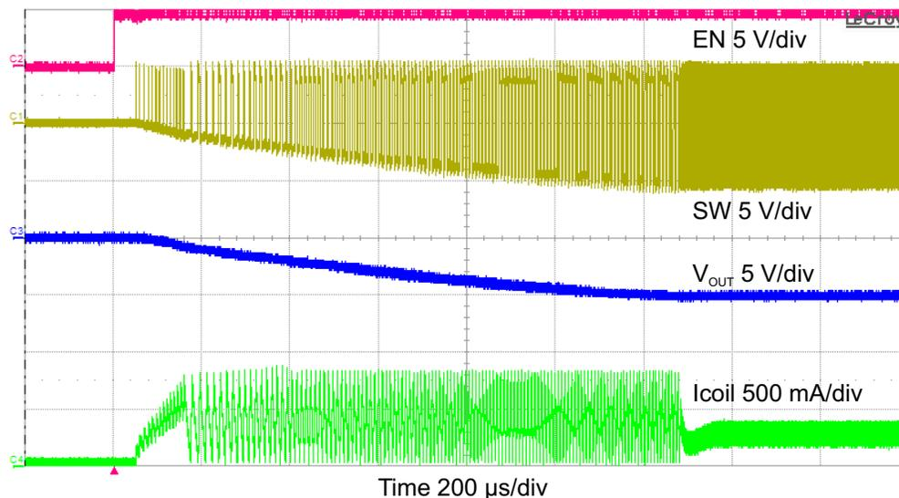
**Figure 13. Startup Behavior in the Inverting Configuration with  $V_{IN} = 5$  V and 120-mA load**
