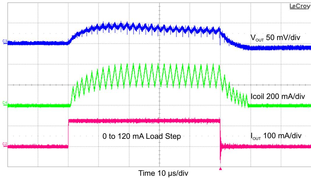
Figure 20. Load Transient Response with  $V_{IN} = 5\text{ V}$
