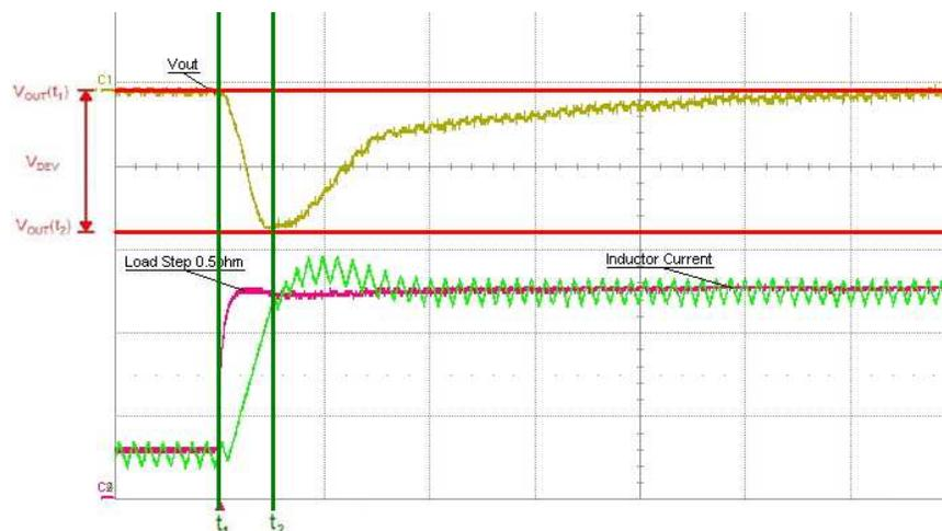
Figure 1. Load Transient Response of the TLV62090
