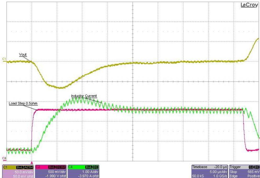
Figure 3. Load Transient with 2.2-µH Inductor and 100-µF Capacitor
