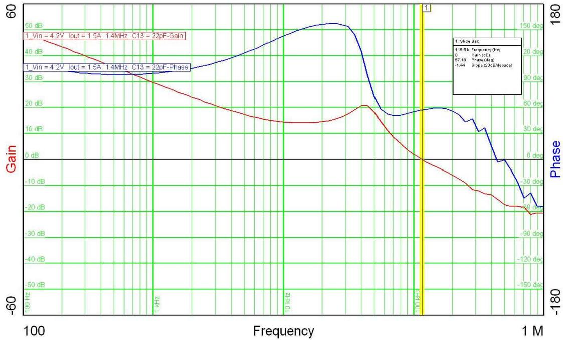
Figure 4. Control Loop Gain with 2.2- $\mu$ H Inductor and 10- $\mu$ F Capacitor
