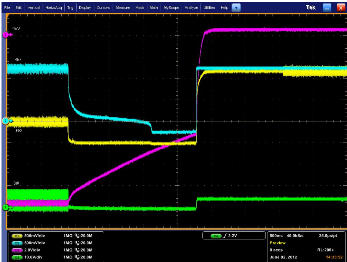
Figure 10. REF pin drops 270mV below GND and device does not startup properly
