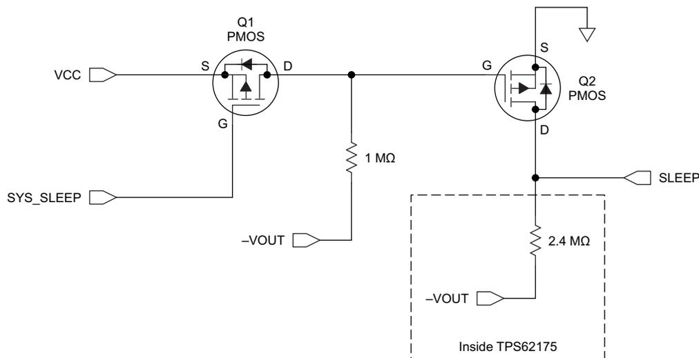
**Figure 7. SLEEP Pin Level Shifter**
