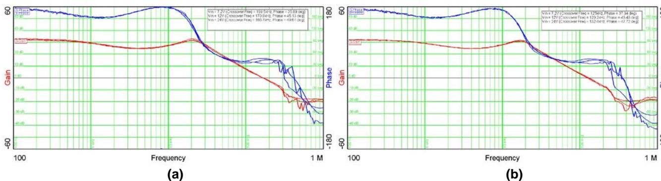
Figure 2. TPS62175 Closed-Loop Frequency Response Using a
