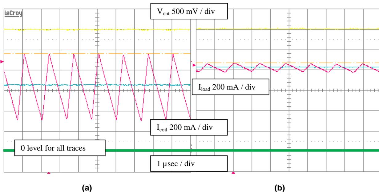
Figure 4. TPS62175 Maximum Output Current Using a (a) 4.7-μH and (b) 47-μH Inductor
