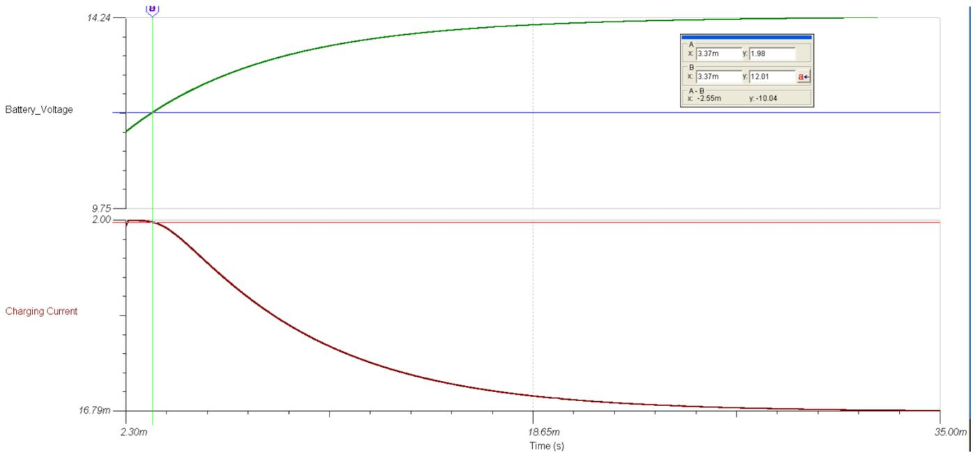
The initial condition assumed it that the battery is in a discharged mode. As observed, the CC Mode lasts till the 12V zener breaks down. At 12V, the CV Mode beings and the current begins to reduce. The voltage builds to  $V_z = 12V + 2.5V$  due to the resistor network of R4 and R5.
