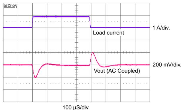
Figure 8. Figure 1 Circuit Load Transient Response
