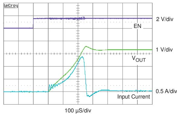
**Figure 2. TPS63010EVM With Extra Output Capacitance Soft Starting Into 100-Ω Load – 250-μs Soft Start Time and 1.4 A of Inrush Current**
