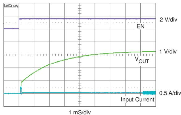
**Figure 3. Figure 1 Circuit Soft Starting Into 100-Ω Load – 8-mS Soft Start Time and 300 mA of Inrush Current**
