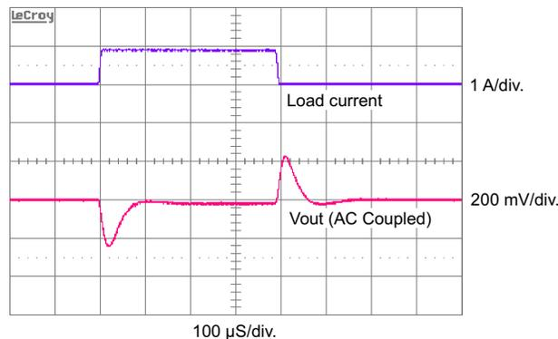
Figure 7. TPS63010EVM Load Transient Response With Extra Output Capacitance but Without Soft Start Circuit
