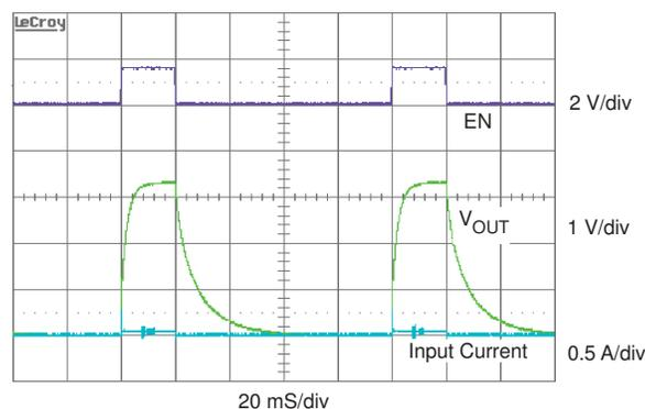
Figure 6. Figure 5 Circuit With EN Toggling at 10 Hz and 20% Duty Cycle – 300 mA of Inrush Current
