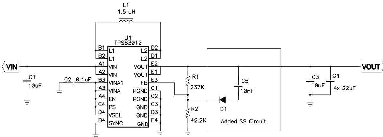
Figure 1. TPS63010EVM With Added Soft Start Circuit
