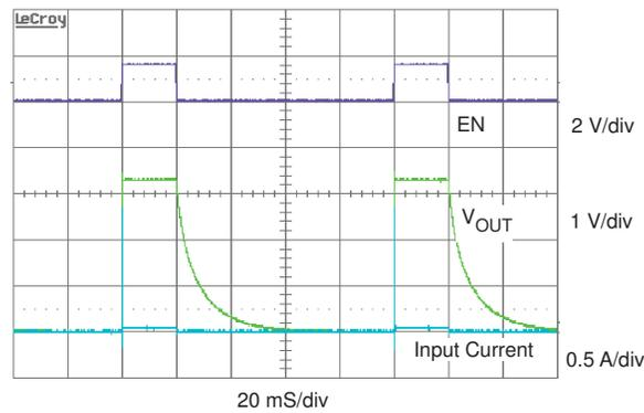
Figure 4. Figure 1 Circuit With EN Toggling at 10 Hz and 20% Duty Cycle – 1.4 A of Inrush Current
