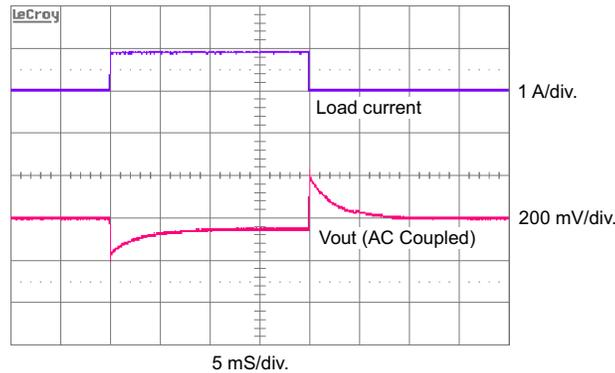
**Figure 9. Figure 5 Circuit Load Transient Response**
