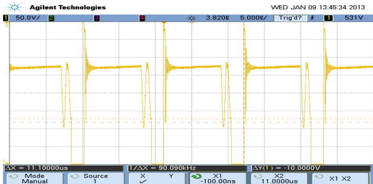
Figure 6. Switch Node Waveform, Normal Operating Condition, 0% Dimming (Frequency of Operation = 90 kHz)
