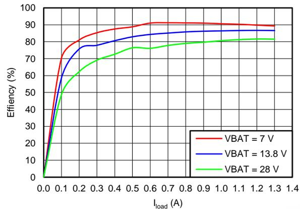
Figure 2. Efficiency Results VDD6 BUCK
