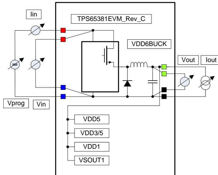
Figure 1. Efficiency Test Setup for VDD6 BUCK
