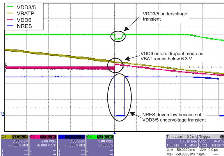
Figure 1. Battery Slow Ramp-Down Bench Measurement Result
