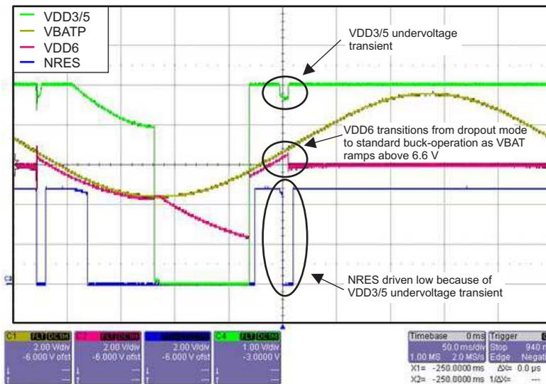
Figure 3. Battery Slow Ramp-Up Bench Measurement Result
