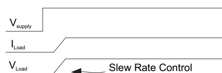
Figure 7. Slew Rate Control with Load Switch
