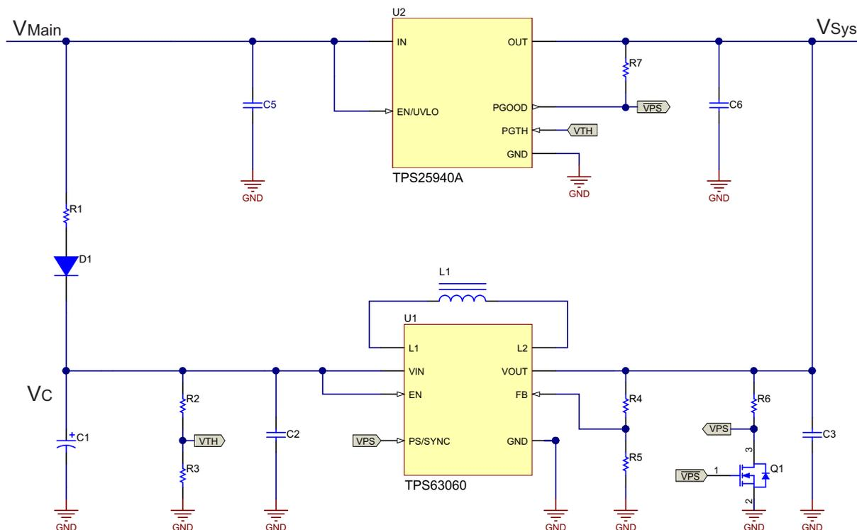
**Figure 2. SSD Backup Power Application Schematic**
