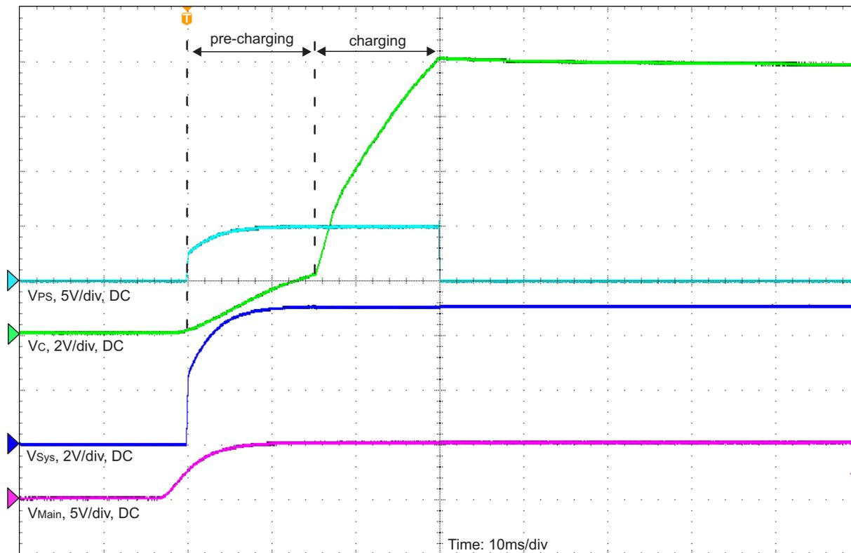
Figure 5. Pre-Charging and Charging of the Backup Capacitor
