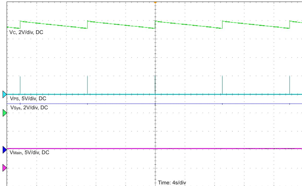
**Figure 7. Normal Operation (Recharge Cycles)**
