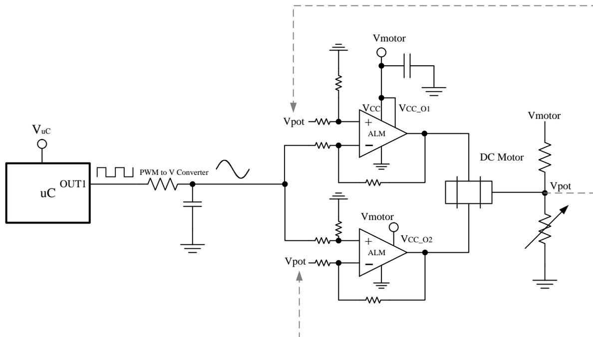
**Figure 11. ALM2402Q1 Used as a Servo Motor Driver**
