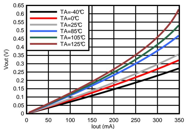
Figure 3. Output Low (VOL) vs. Temperature
