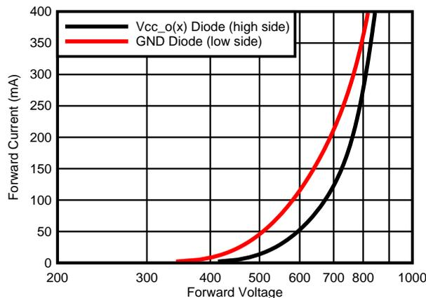
**Figure 9. PMOS (High Side) & NMOS (Low Side) Output Diode Forward Voltage**
