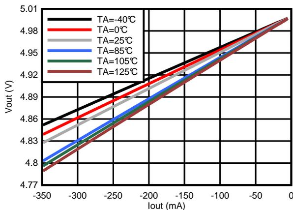
Figure 2. Output High (VOH) vs. Temperature
