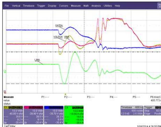
**Figure 9.  $V_{IN}$  Transient Generated by  $V_{BIAS} = 25$  V and  $C_{GLITCH} = 100$  nF**
