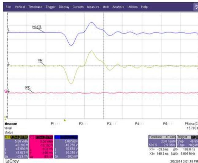
Figure 10. Mechanical Glitch With a 1- $\mu\text{F}$   $C_{OUT}$
