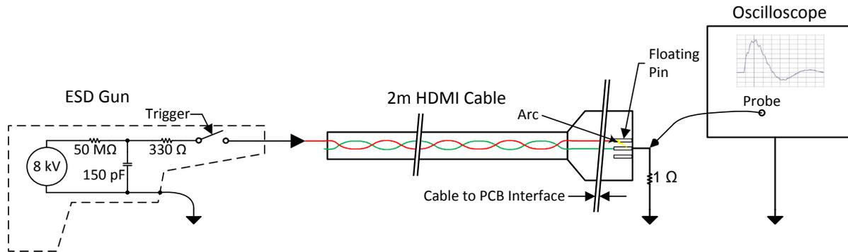
**Figure 2. Test Setup for Capturing the EOS Waveform**
